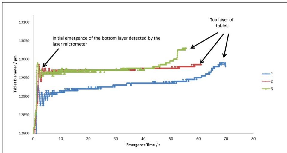
Fig. 8: Tablet diameter versus emergence time during the ejection of bi-layered tablets with MCC as bottom layer (22.6 MPa) and lactose as top layer (46.21 MPa).
