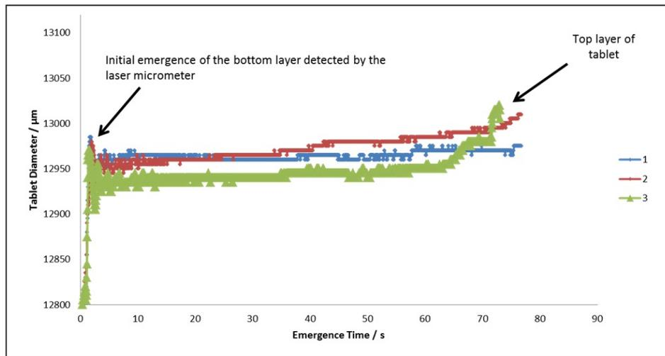
Fig. 7: Tablet diameter versus emergence time during the ejection of bi-layered tablets with MCC as bottom layer (22.6 MPa) and lactose as top layer (22.6 MPa).
