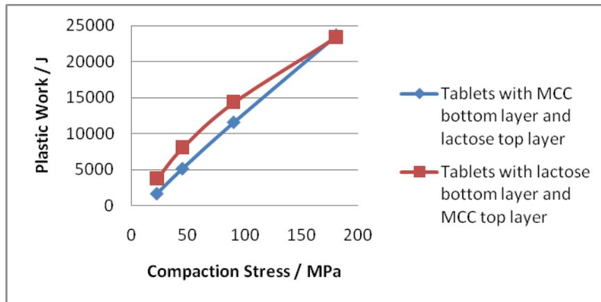
Fig.4: Plastic work at different compaction stresses.
