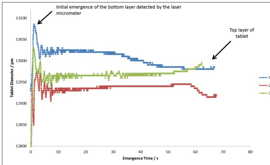
Fig. 12: Tablet diameter versus emergence time during the ejection of bi-layered tablets with lactose as bottom layer (22.6 MPa) and MCC as top layer (46.21 MPa).
