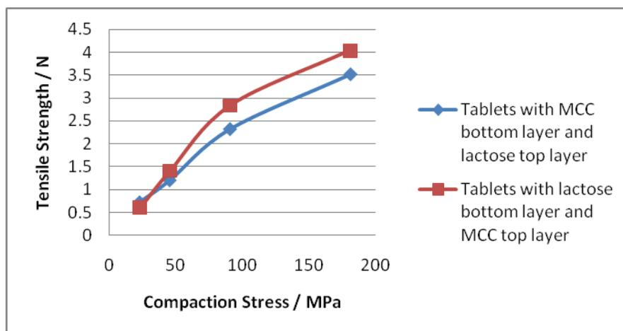
Fig. 15: Tensile strength of bi-layered tablets at different compaction stresses.
