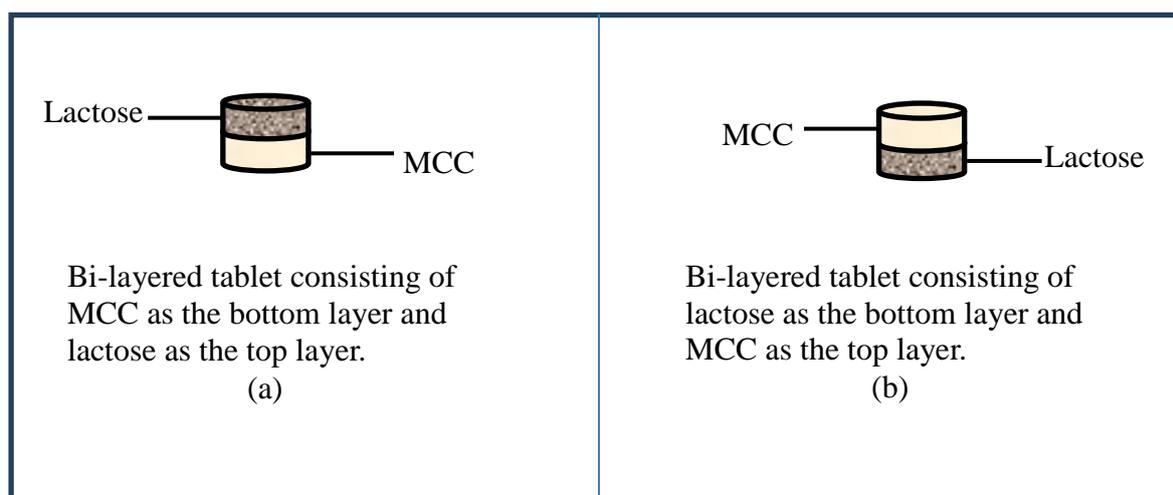
Fig. 3: Bi-layered tablet compositions produced in this study: (a) MCC as bottom layer and lactose as top layer; (b) lactose as bottom layer and MCC as top layer.
