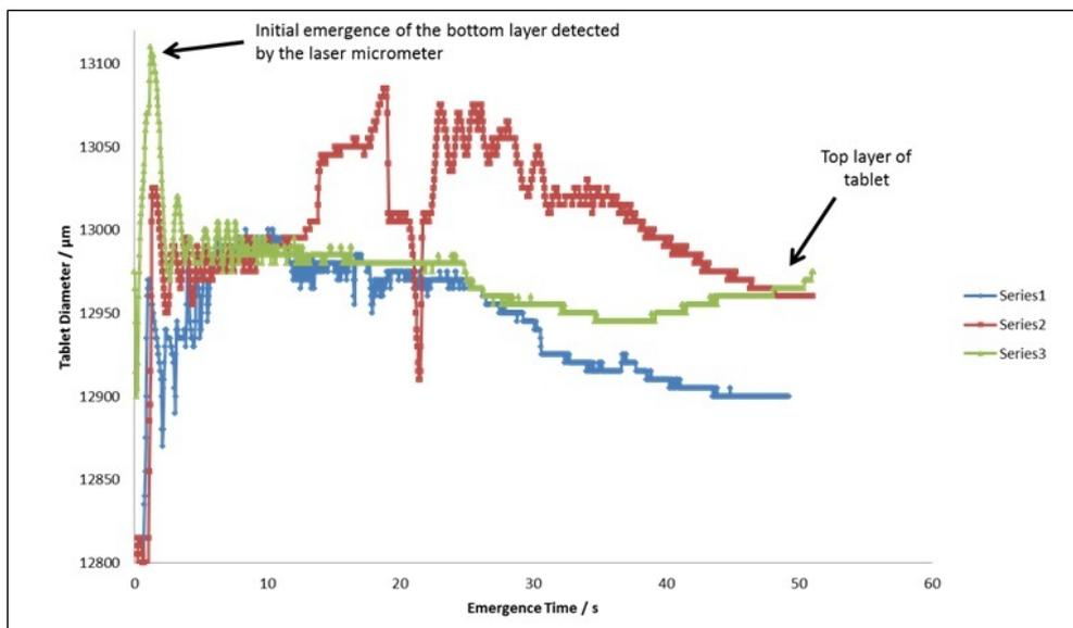
Fig. 14: Tablet diameter versus emergence time during the ejection of bi-layered tablets with lactose as bottom layer (22.6 MPa) and MCC as top layer (180.86 MPa).
