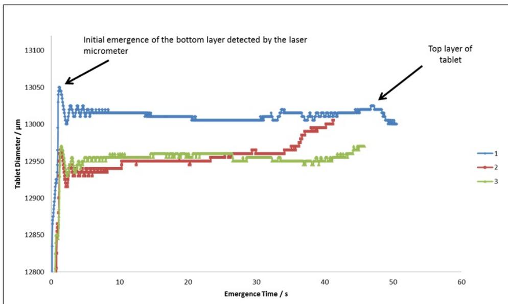
Fig. 10: Tablet diameter versus emergence time during the ejection of bi-layered tablets with MCC as bottom layer (22.6 MPa) and lactose as top layer (180.86 MPa).
