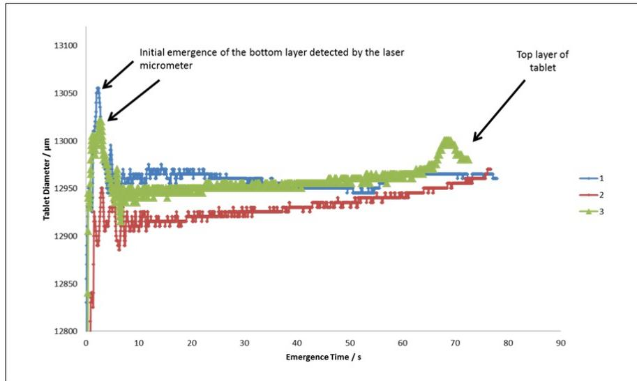
Fig.11: Tablet diameter versus emergence time during the ejection of bi-layered tablets with lactose as bottom layer (22.6 MPa) and MCC as top layer (22.6 MPa).
