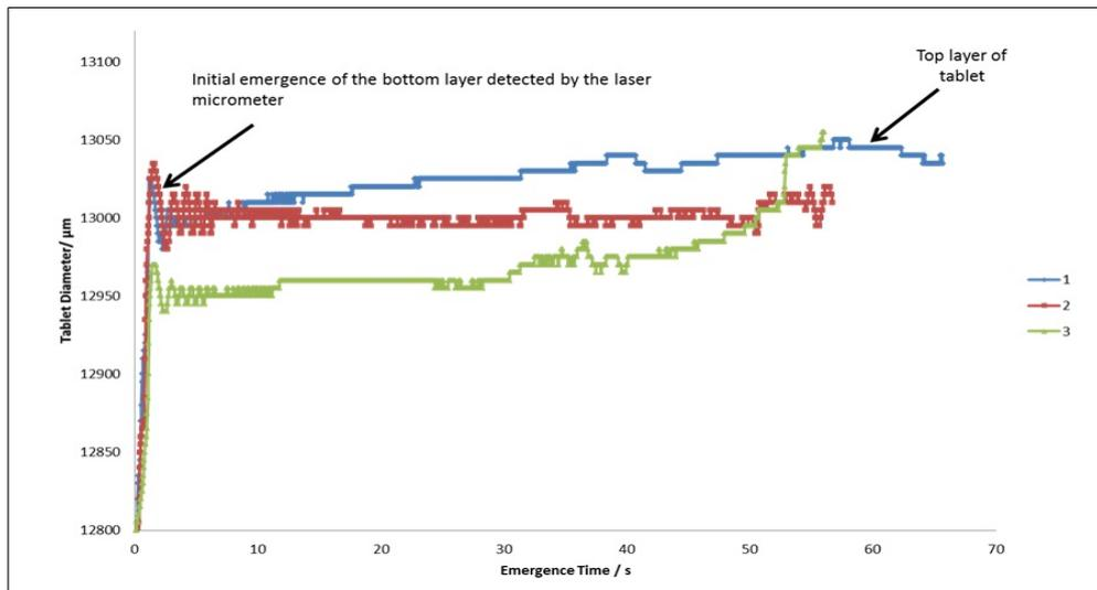
Fig. 9: Tablet diameter versus emergence time during the ejection of bi-layered tablets with MCC as bottom layer (22.6 MPa) and lactose as top layer (90.43 MPa).
