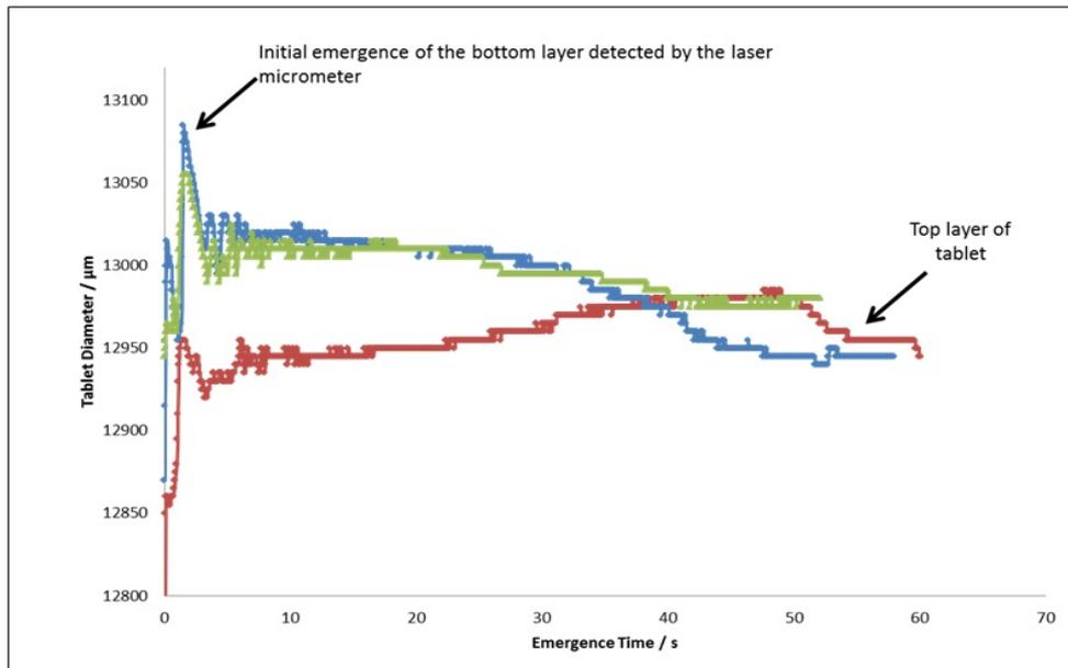
Fig. 13: Tablet diameter versus emergence time during the ejection of bi-layered tablets with lactose as bottom layer (22.6 MPa) and MCC as top layer (90.43 MPa).
