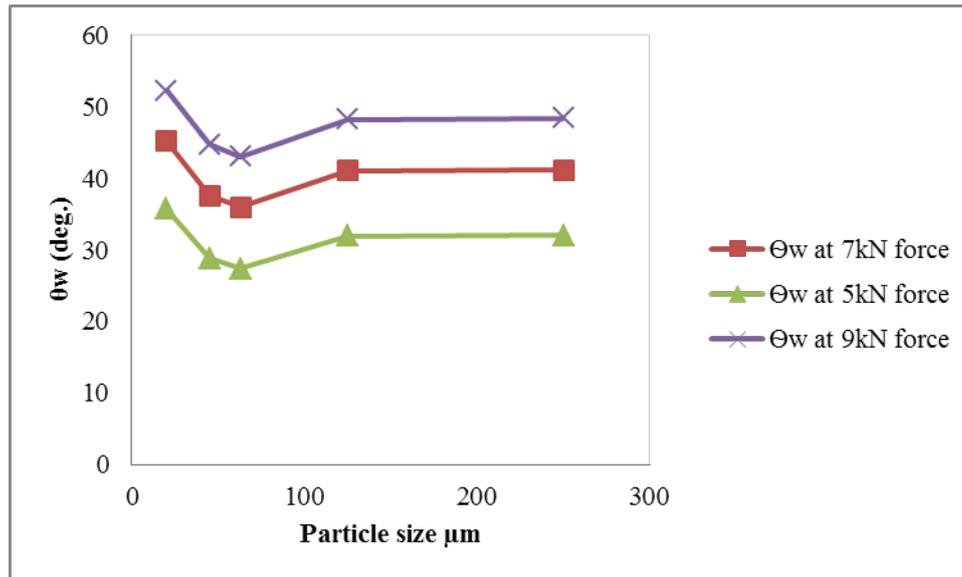
Fig 2: Wall friction angle versus particle size at different applied loads upon uniform weight of *Labisia pumila* powder extracts.
