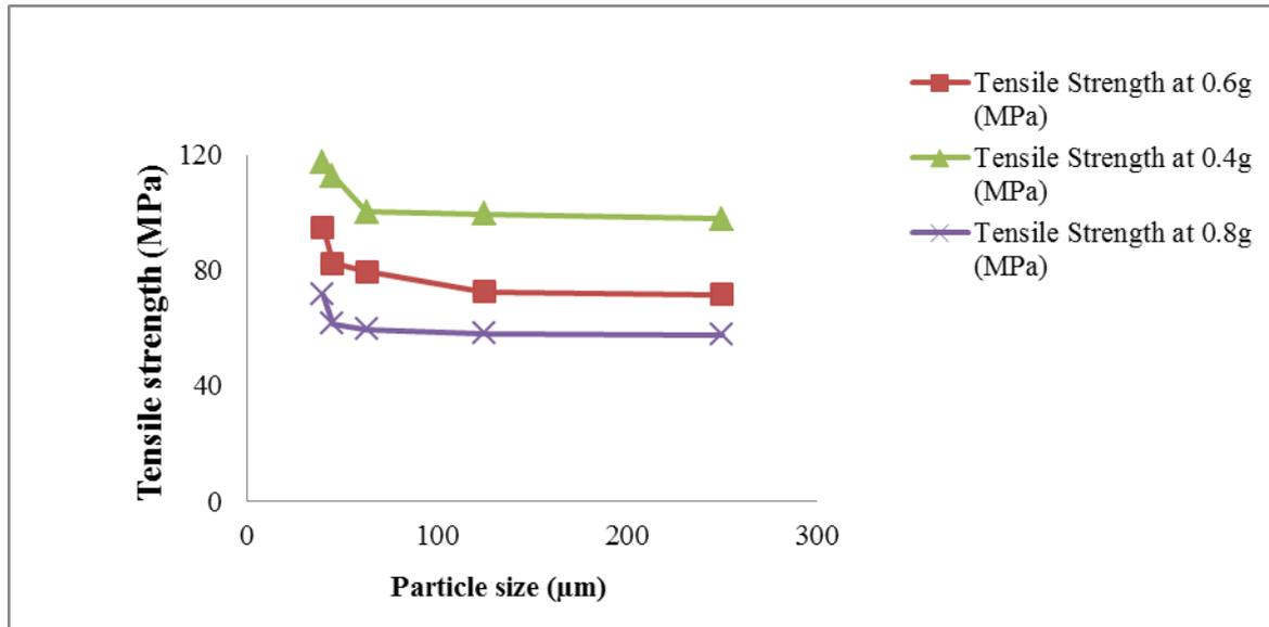
Fig 4 : Particle size versus Tensile strength of *Labisia pumila* powder at different weights upon uniform load.
