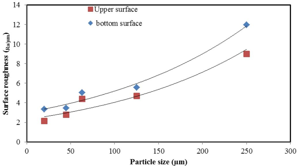
Fig 1: The trend lines of Surface roughness  $R_a$  versus particle size for 0.8g of compacted *Labisia pumila* powder.
