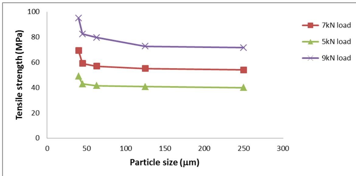
Fig 5: Particle size versus Tensile strength of *Labisia pumila* powder at different loads upon uniform weight. Particle size
