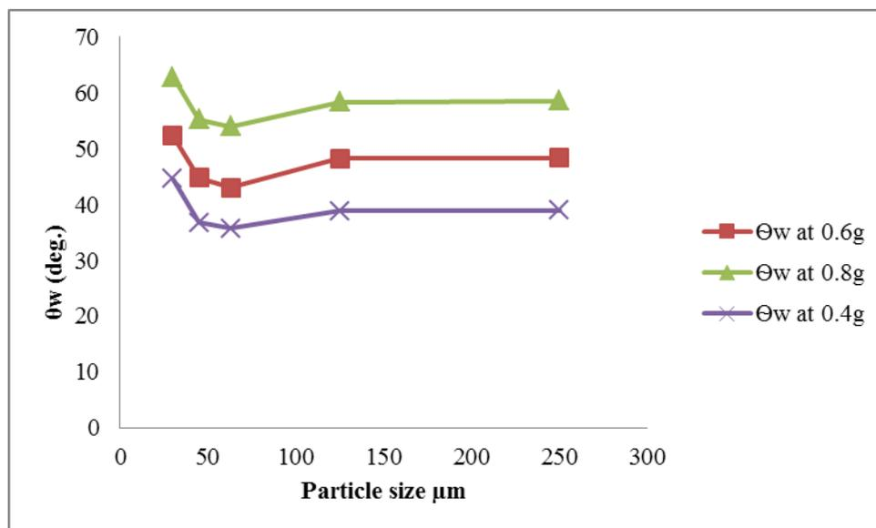
Fig 3: Wall friction angle versus particle size at uniform applied load upon different weight of *Labisia pumila* powder extracts.
