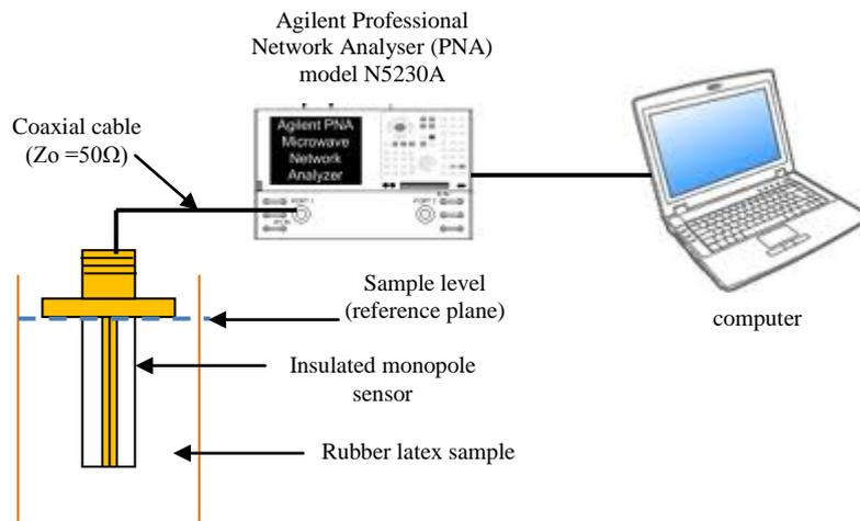
Fig. 2: The measurement set-up
