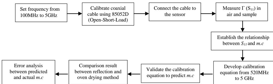
Fig. 1: The procedure of reflection measurement ( $S_{11}$ )
