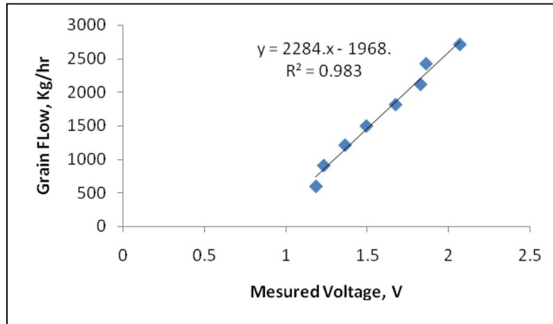
Fig. 7: Calibration graph for microwave solid flow sensor.
