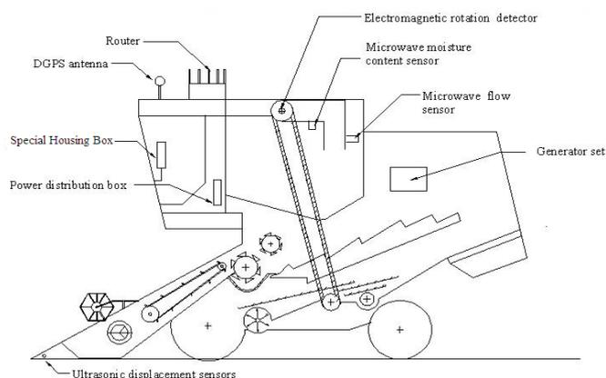
Fig 2: Locations of the various units of the instrumentation system.
