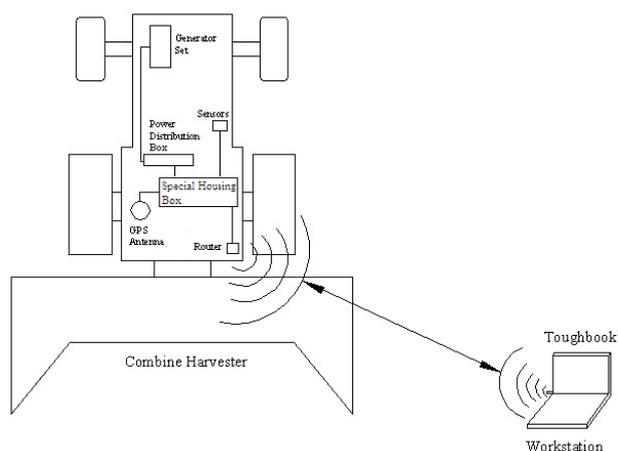
Fig 1: Simplified diagram of the complete instrumentation system.
