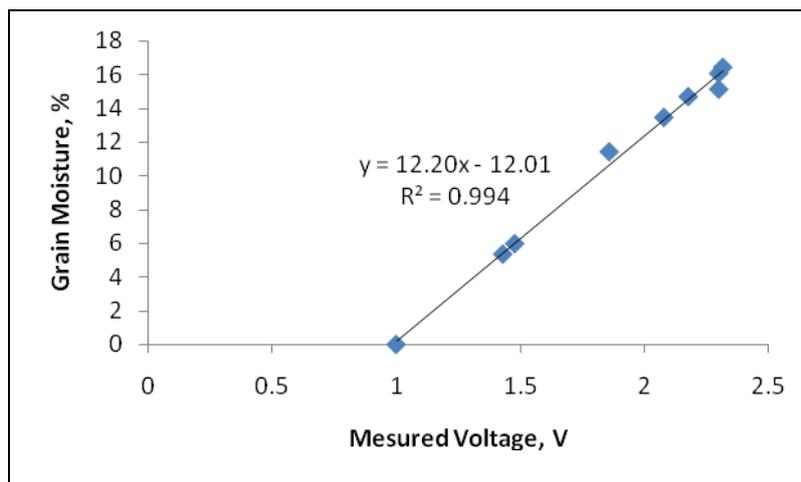
Fig. 8: Calibration graph for microwave moisture sensor.
