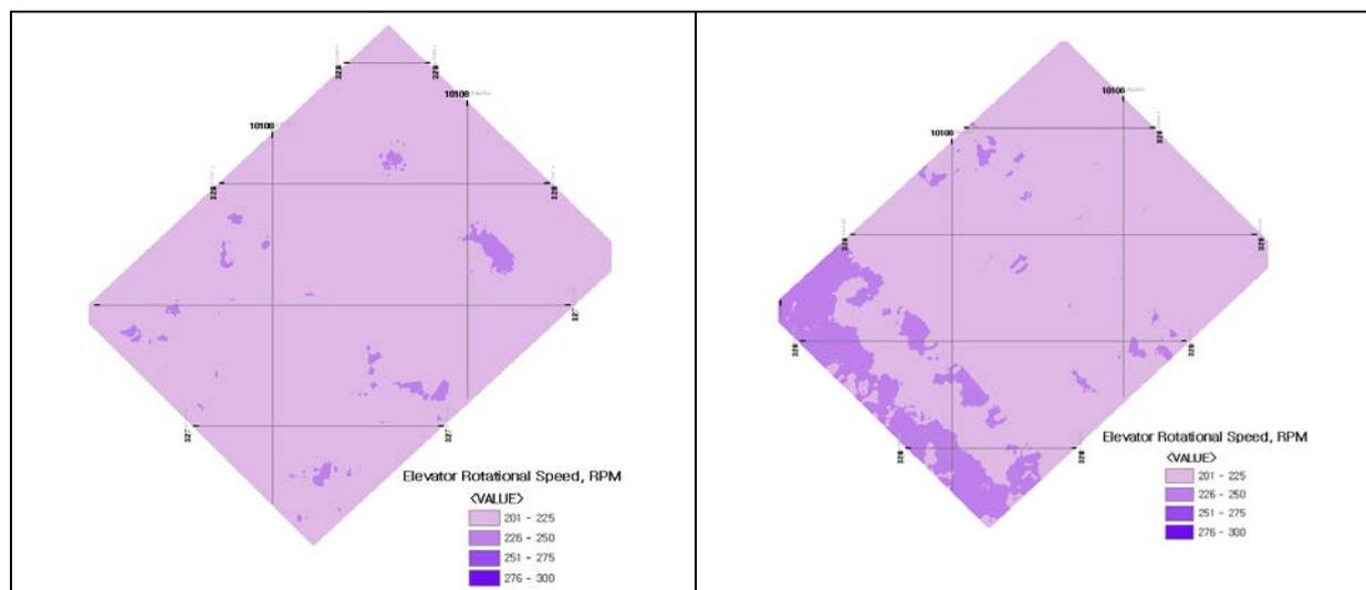
Fig. 16: Combine elevator rotational speed maps for lots T0 and T1.
