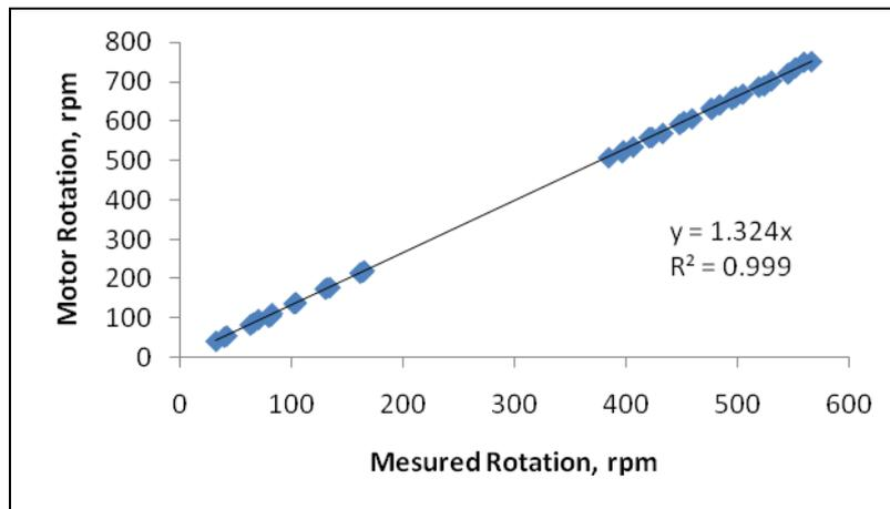
Fig. 6: Calibration graph for electronic rotation detector.
