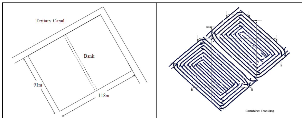
Fig. 9: Field layout and combine tracking map for lot T0.
