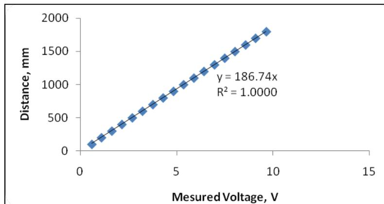
Fig. 5: Calibration graph for ultrasonic displacement sensor.
