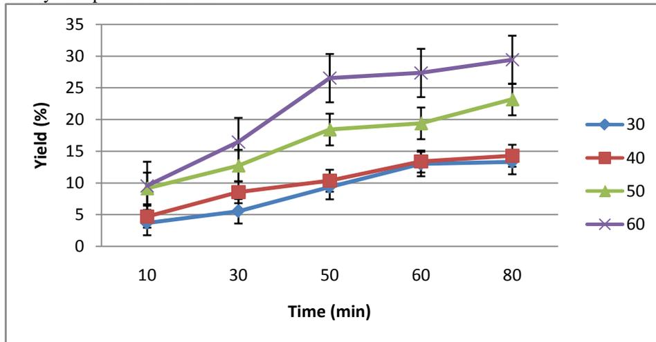
Fig. 3 (a): Effect temperature for palm fruit at 1 hour reaction time, 476:1 ethanol to oil molar ratio and 0.1 mol catalyst concentration
