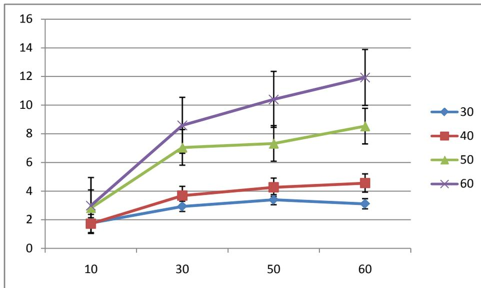
Fig. 3 (b): Effect temperature for waste mesocarp at 1 hour reaction time, 576:1 ethanol to oil molar ratio and 0.1 mol catalyst concentration
