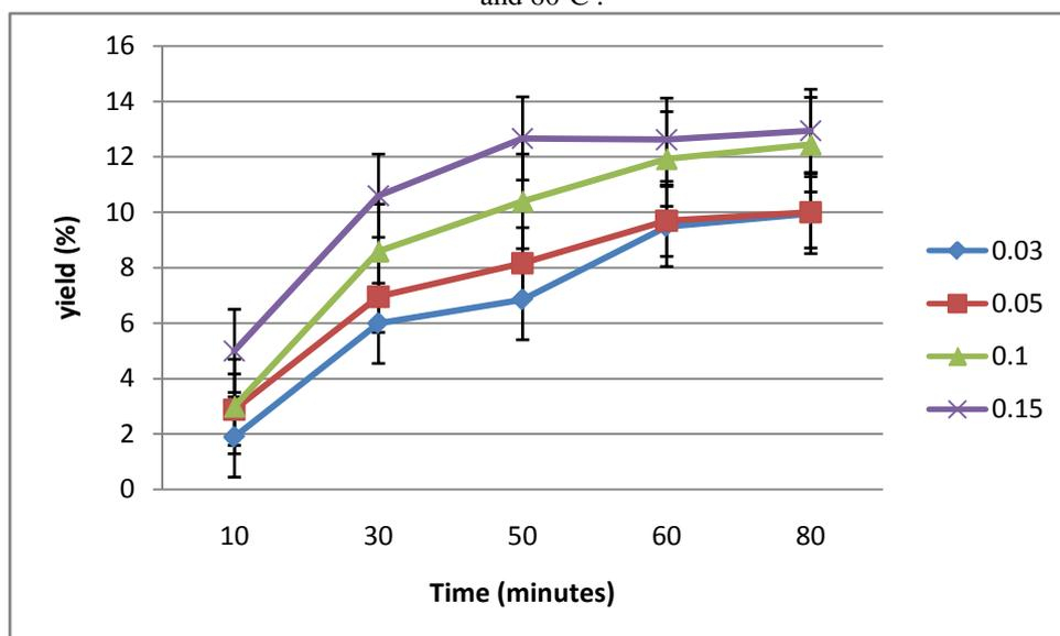
Fig. 2 (b): Effect of catalyst concentration for waste mesocarp at 1 hour reaction time, 576:1 ethanol to oil molar ratio and 60°C .
