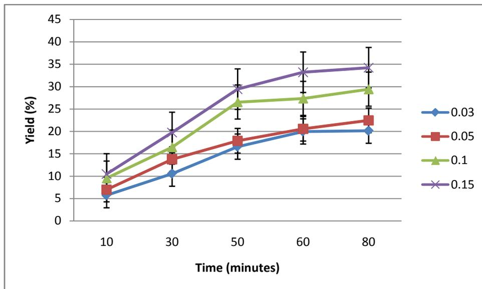
Fig. 2 (a): Effect catalyst concentration for palm fruit at 1 hour reaction time, 476:1 ethanol to oil molar ratio and 60°C .
