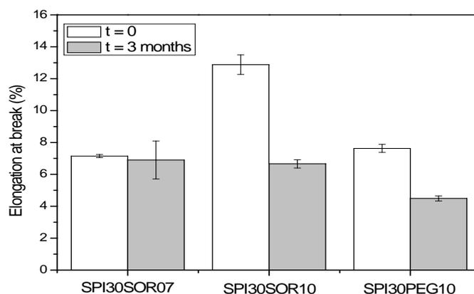
Fig. 5: Elongation at break of the SPI-based films prepared in this study.
