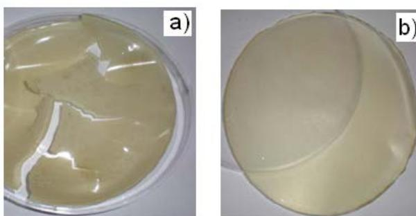
Fig. 1: Visual aspect of a) SPI20SOR10 and b) SPI30SOR10 films.
