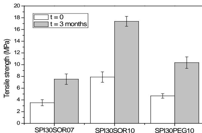
Fig. 4: Tensile strength of the SPI-based films prepared in this study.
