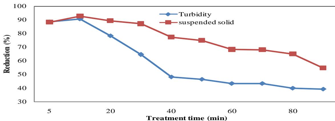
Fig. 2: Effect of treatment time on turbidity and suspended solid using CSC adsorbent. Adsorbent dose: 20g/l, pH: 4.2, and stirring speed: 150 rpm.
