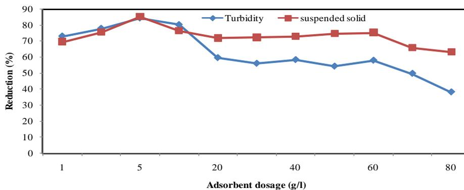
Fig. 3: Effect of adsorbent dose on turbidity and suspended solid using CSC adsorbent. Treatment time: 10 minutes, pH: 4.2 and stirring speed: 150 rpm.
