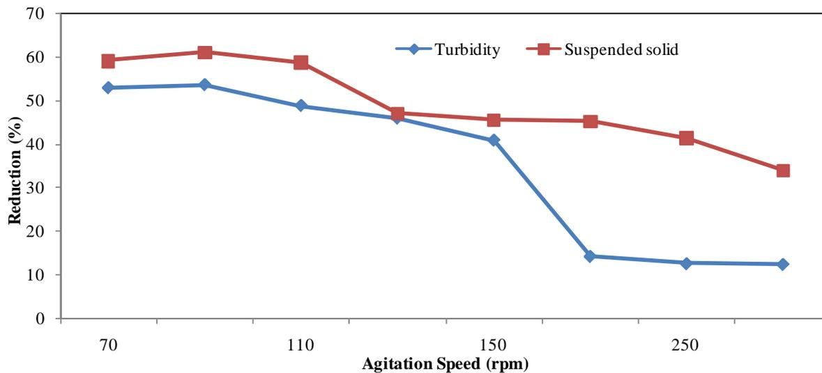
Fig. 6: Effect of agitation speed on turbidity and suspended solid using CSC adsorbent. Treatment time: 10 minutes, Adsorbent dose: 5g/l and pH: 4.2.
