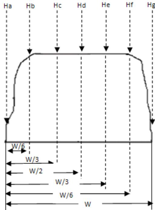
Fig. 7: Height measurements for describing the cross sectional area of the compost heap.
