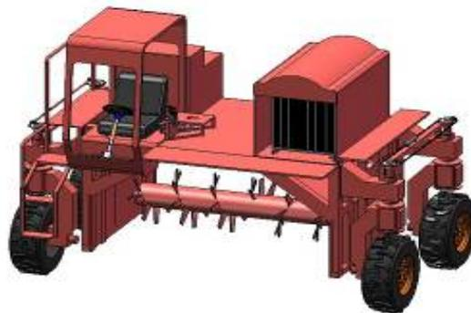
Fig. 2: 3-D CAD of the developed self-propelled turning machine.
