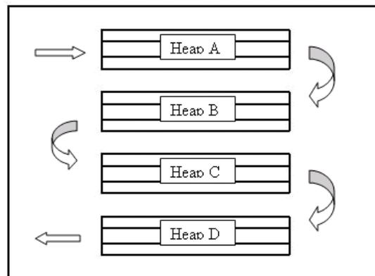
Fig. 4: Machine movements during the turning operation on the compost heaps.
