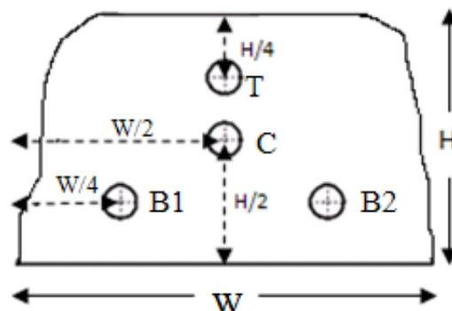
Fig. 6: Sampling points for temperature and oxygen content measurements in the compost heap.
