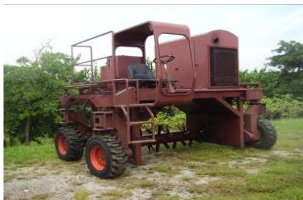
Fig. 3: Picture of the prototype self-propelled turning machine.
