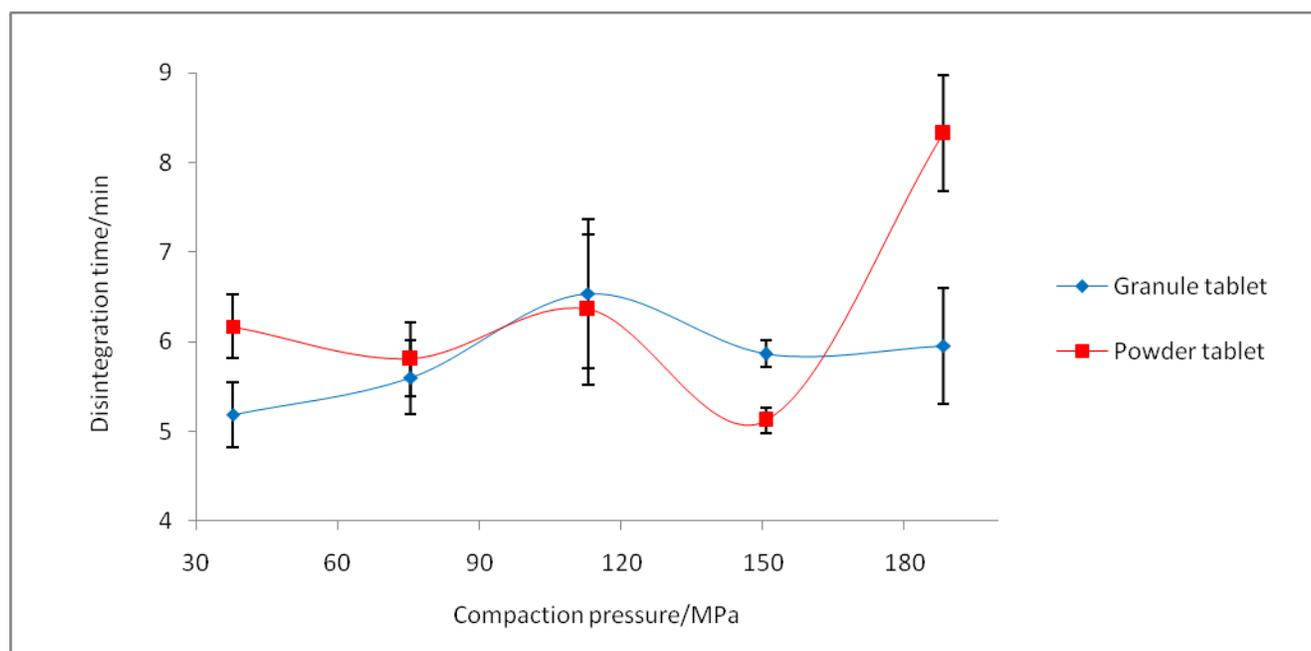
Fig. 8: Disintegration rate of urea in powder and granule form at various compaction pressures. (Standard errors are indicated by error bars)
