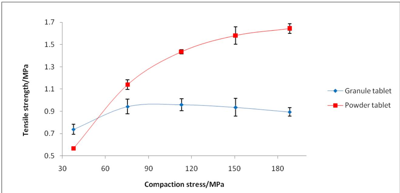
Fig. 7: Tableability of urea in powder and granule form at various compaction pressures. (Standard errors are indicated by error bars)
