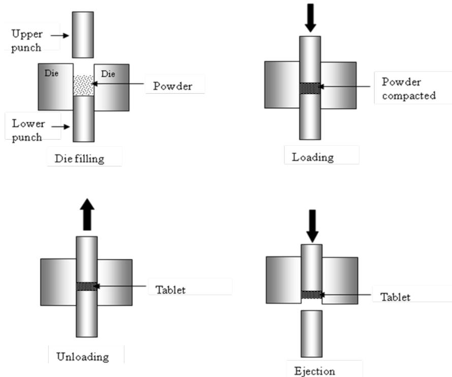
Fig. 3: Compaction cycle [7].
