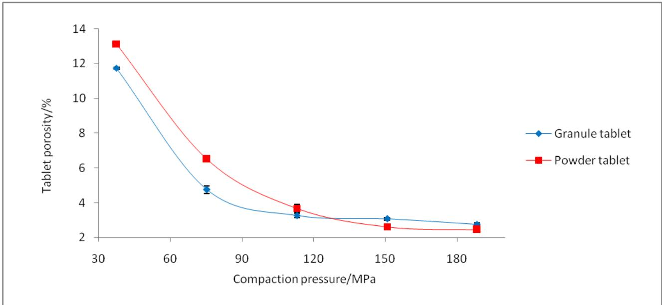
Fig. 5: Compressibility of urea powder and granule at various compaction pressures. (Standard errors are indicated by error bars)
