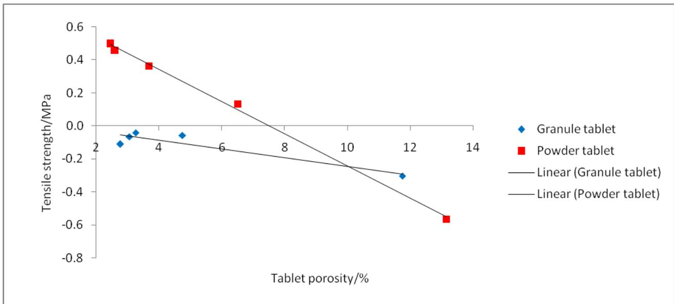
Fig. 6: Compactibility of urea in powder and granule form at various compaction pressures. (Standard errors are indicated by error bars).
