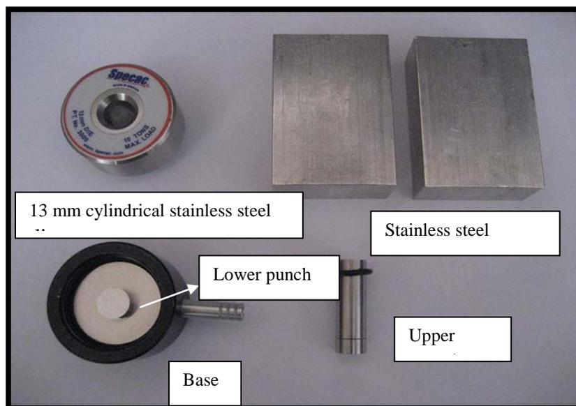
Fig. 4: 13 mm stainless steel cylindrical uniaxial die
