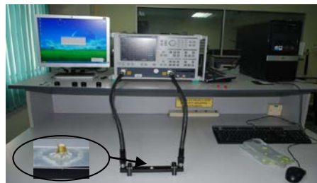
Fig. 3: The Vector Network Analyzer with Kenaf sample inside the Rectangular
