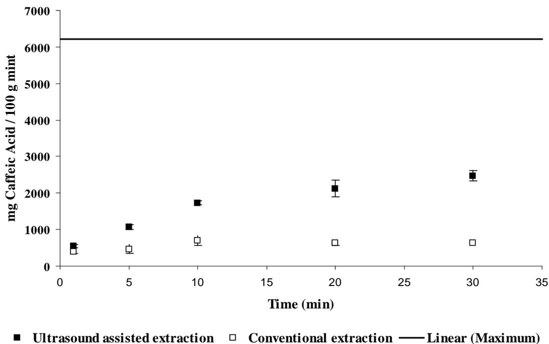
Fig. 4: Effect of extraction time of ultrasound assisted extraction and conventional extraction on hydroxycinnamic acid derivatives
