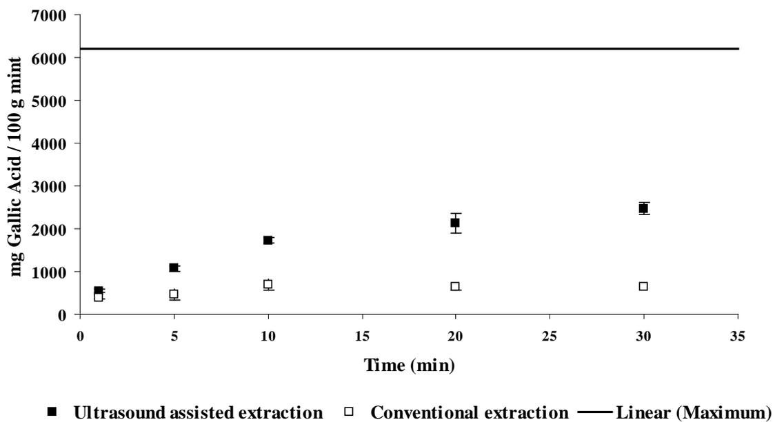
Fig. 3: Effect of extraction time of ultrasound assisted extraction and conventional extraction on estimated phenolic content by (a) Folin-Ciocalteu method and (b) Obied protocol.
