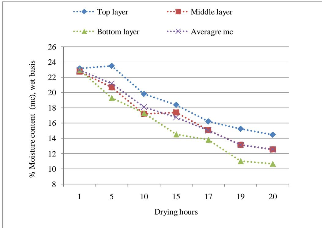
Fig. 3: Drying curve during inclined bed paddy drying.
