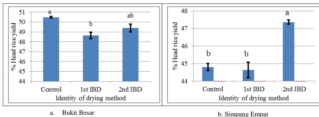
Fig. 8: Comparison of head rice yield obtained from different drying line of the two complexes of BERNAS. [IBD is inclined bed dryer, <sup>a-d</sup> The test values: Same letters for the different drying methods in each figure mean that the values are not significantly different ( $p > 0.05$ )].
