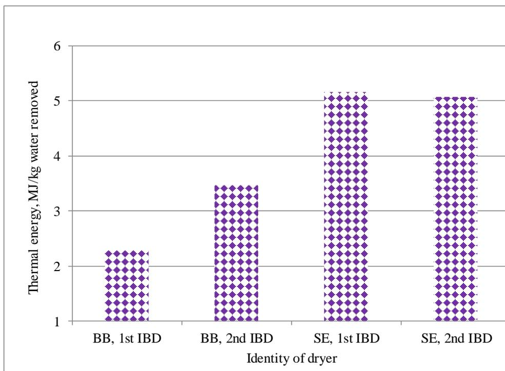
Fig. 6: Thermal energy consumption in paddy drying with inclined bed dryer of the two complexes of BERNAS. [BB: Bukit Besar, SE: Simpang Empat, IBD: inclined bed dryer]
