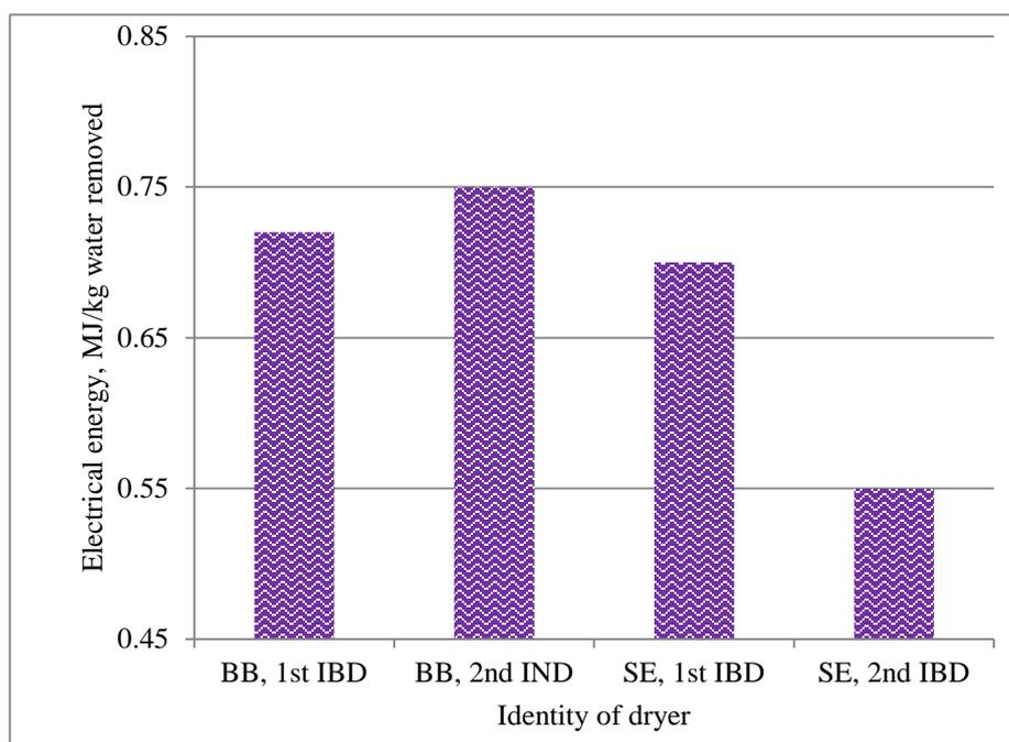
Fig. 7: Electrical energy consumption during paddy drying with inclined bed dryer in the two complexes of BERNAS. [BB: Bukit Besar, SE: Simpang Empat, IBD: inclined bed dryer]
