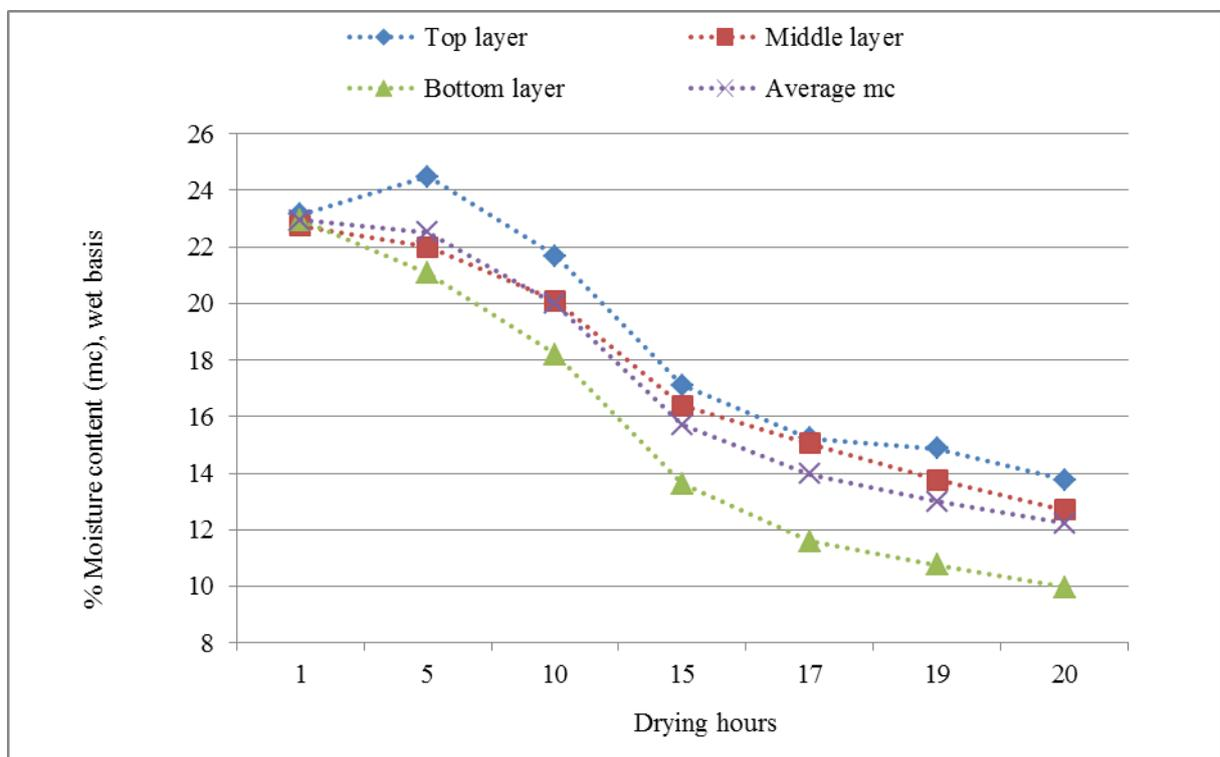
Fig. 2: Drying curve during inclined bed paddy drying.
