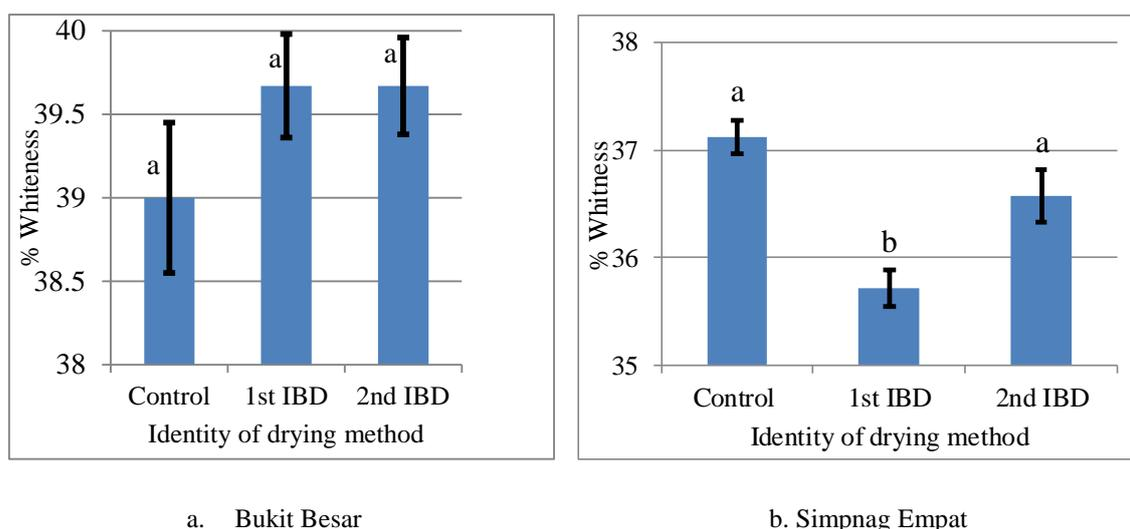
Fig. 9: Comparison of whiteness of rice obtained from different drying lines of two complexes of BERNAS. [IBD is inclined bed dryer, <sup>a-d</sup> The test values: Same letters for the different drying methods in each figure mean that the values are not significantly different ( $p > 0.05$ )].
