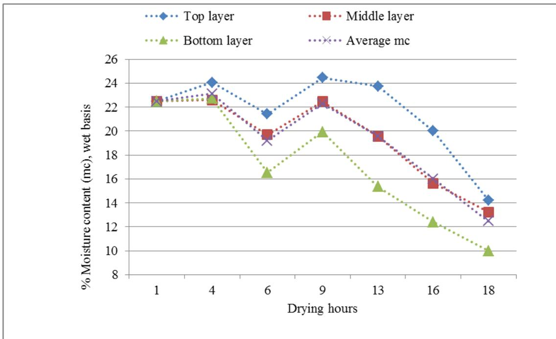
Fig. 4: Drying curve during inclined bed paddy drying.
