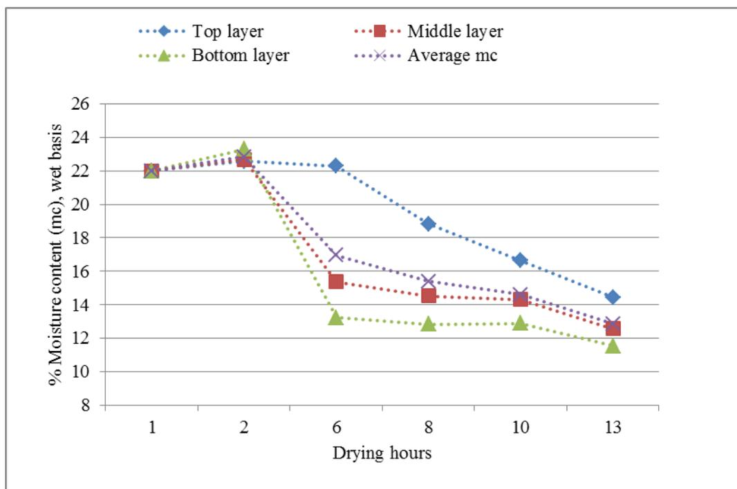
Fig. 5: Drying curve during inclined bed paddy drying.
