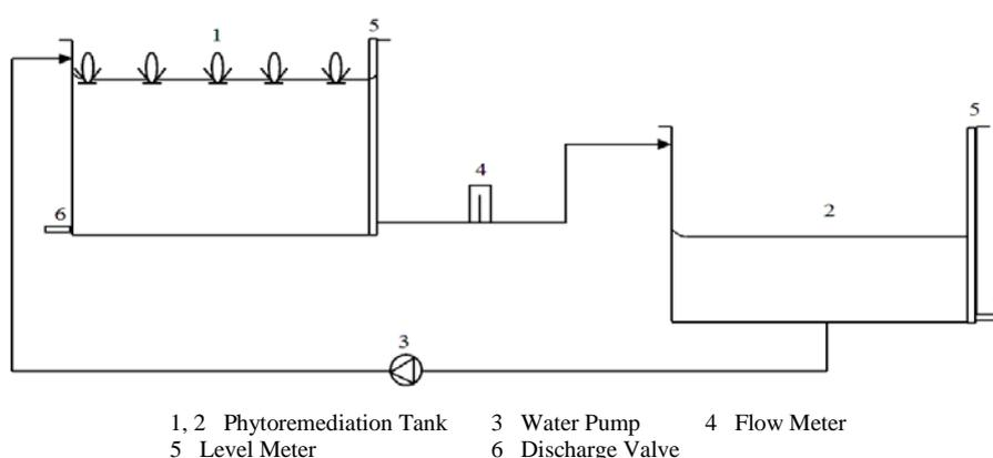
Fig. 1: Schematic diagram of the phytoremediation system
