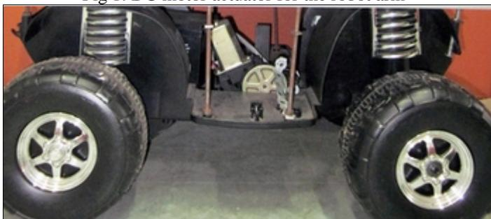
Fig. 3: DC motor driving actuators connected to the robot wheels
