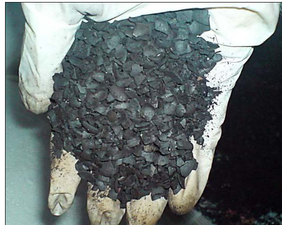
Fig. 3: Oil palm shells after carbonization process
