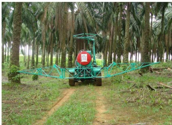
Fig. 6: Prototype universal prime mover with herbicide blanket spraying attachment.
