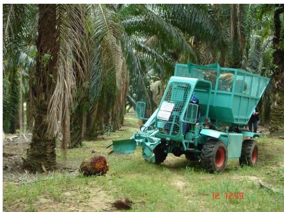
Fig. 7: Prototype universal prime mover with in-field FFB collection-transportation attachment.
