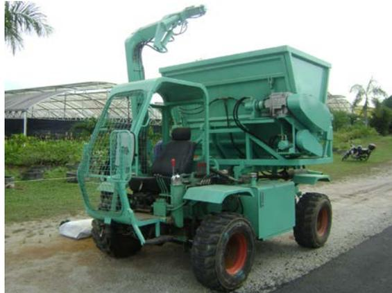
Fig.2: Prototype universal prime mover with soil bagging attachment.
