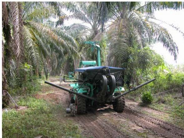
Fig. 4: Prototype universal prime mover with VRT fertilising attachment.
