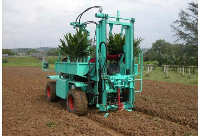
Fig. 3: Prototype universal prime mover with seedling transplanting attachment.
