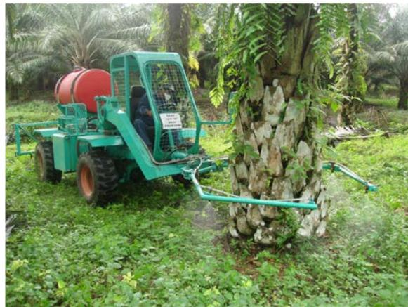
Fig. 5: Prototype universal prime mover with herbicide circle spraying attachment.
