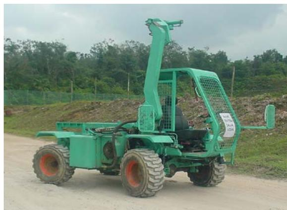
Fig. 1: Prototype universal prime mover.
