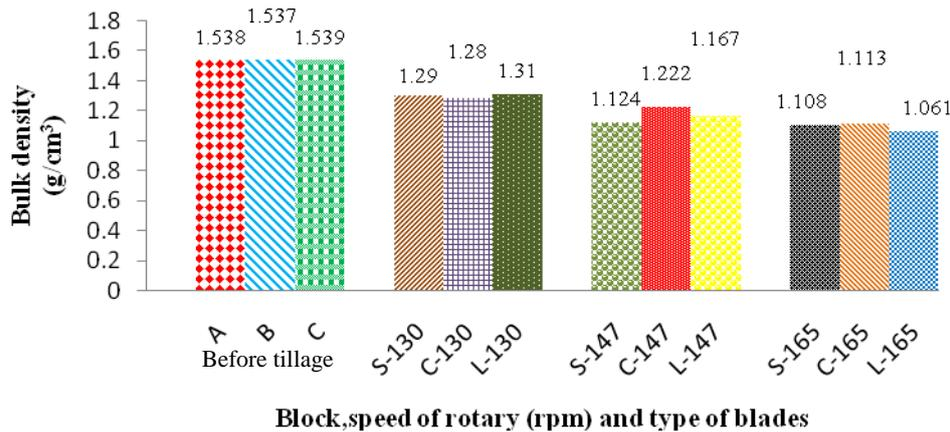
Fig.1: Effect of Blocks, Blade Type and Rotary Speed on Soil Bulk Density (Dry Basis) (S= Straight type blade, C=curved type blade and L= L-shaped blade)
