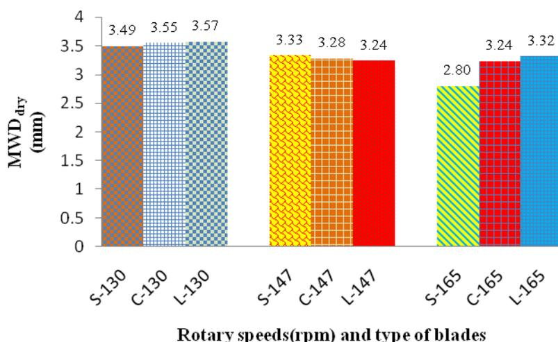
Fig.3: Effect of Blade Type and Rotary Speed on Mean Weight Diameter of Soil Aggregates (Dry Basis) (S= Straight type blade, C=curved type blade and L= L-shaped blade)
