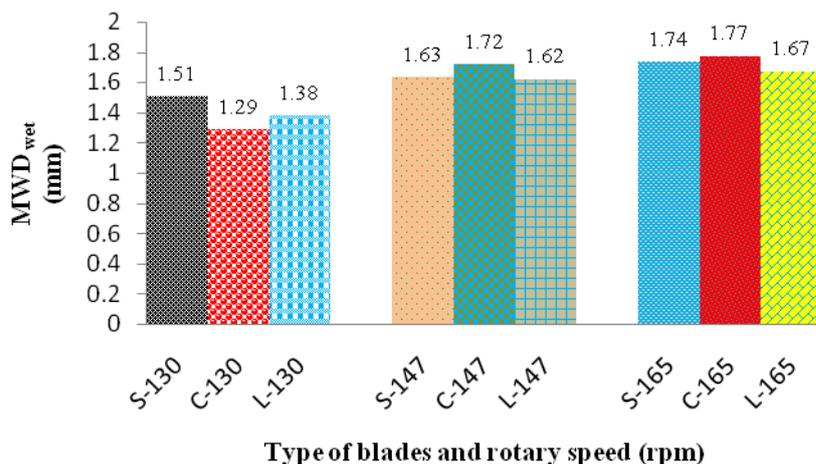
Fig.2: The Effect of Speed of Rotary Blades and Type of Blades on Mean Weight Diameter (Wet Basis) of Soil Aggregates. (S= Straight type blade, C=curved type blade and L= L-shaped blade)
