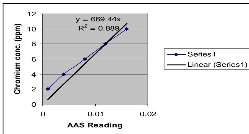
Fig. 5. Standard calibration curve for Chromium
