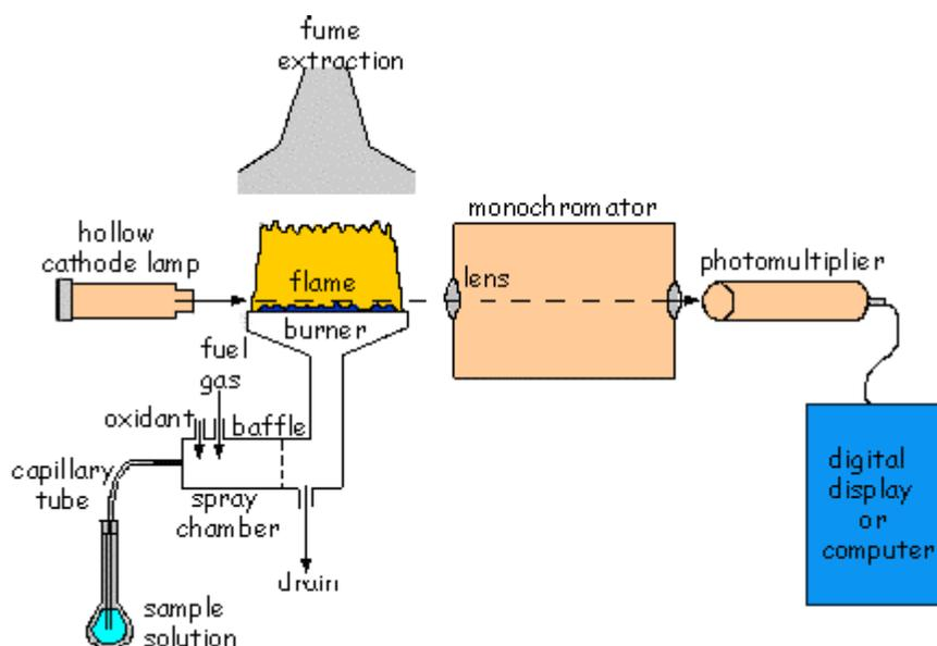
Fig. 1. A schematic diagram of atomic absorption spectrometer
