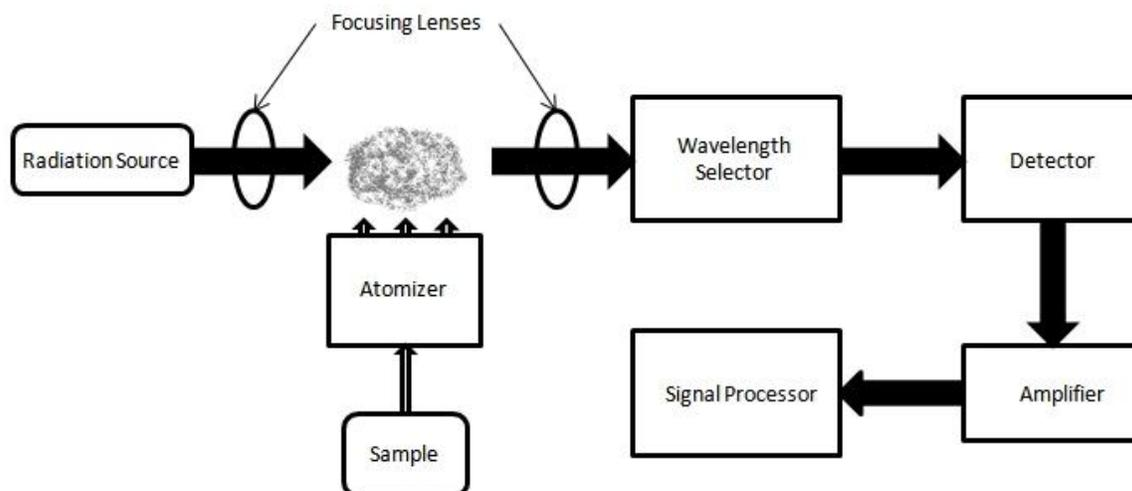
Fig. 2. Atomic absorption spectrometer block diagram (Source:Wikimedia Commons.)
