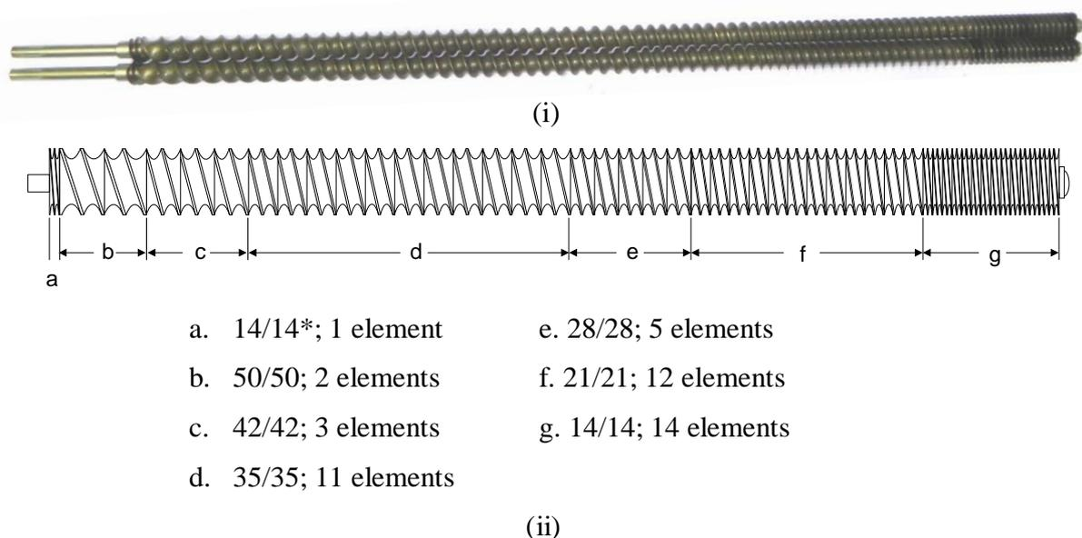
Fig. 1: (i) Photo of the twin screws used in this study, (ii) illustration of the arrangement of the screw elements, not to scale, \*screw element pitch (mm)/length (mm).
