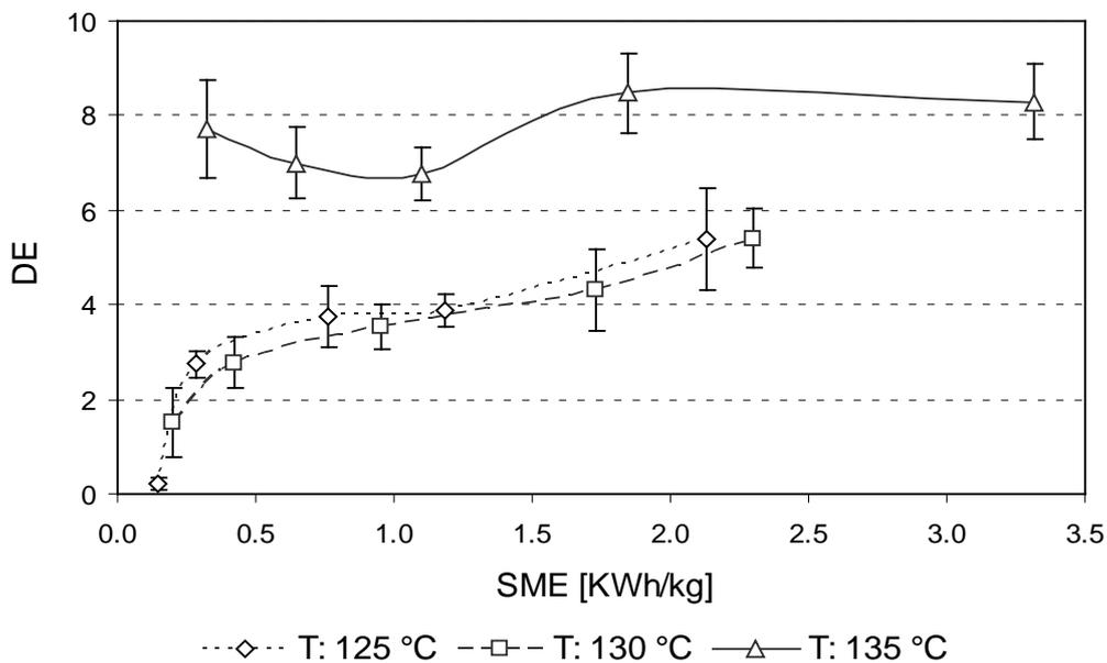
Fig. 9: Effect of specific mechanical energy on the dextrose equivalent of dextrin during extrusion process, vertical and horizontal error bars represent 95% confidence interval.
