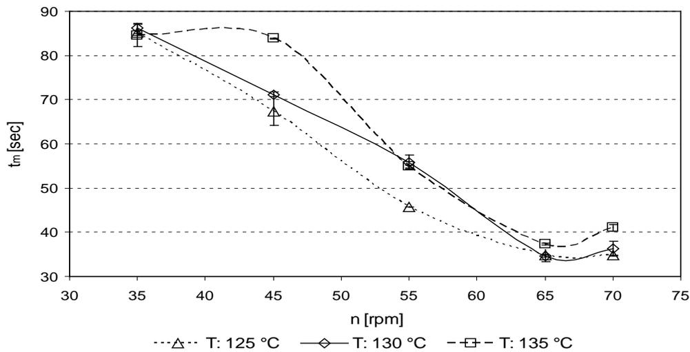
Fig. 3: Mean residence time of acidified corn starch at different screw speed and roasting temperature during the extrusion process, vertical error bars represent 95% confidence interval.
