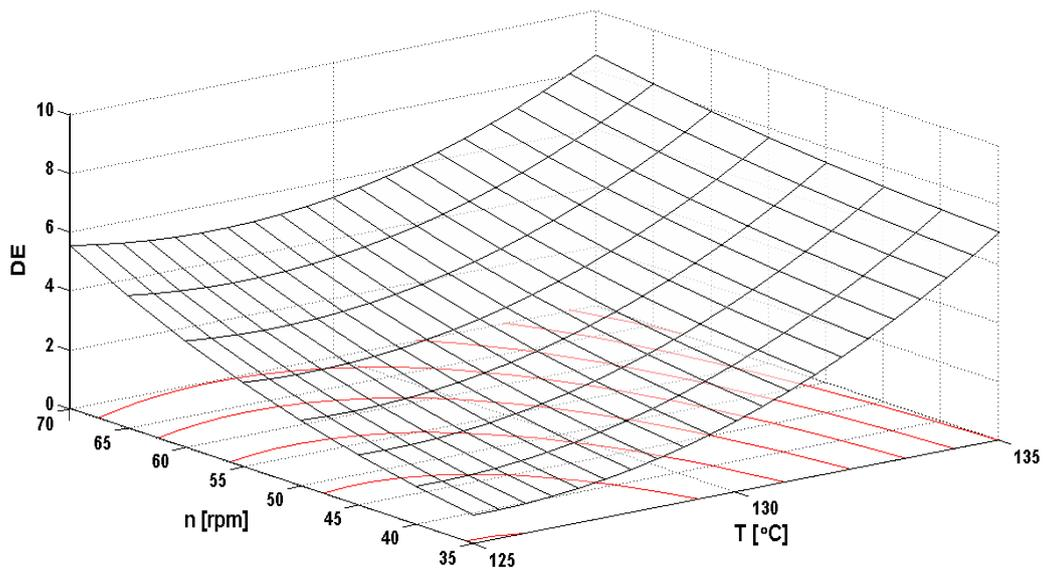
Fig. 2. Effect of screw speed and roasting temperature on the dextrose equivalence value
