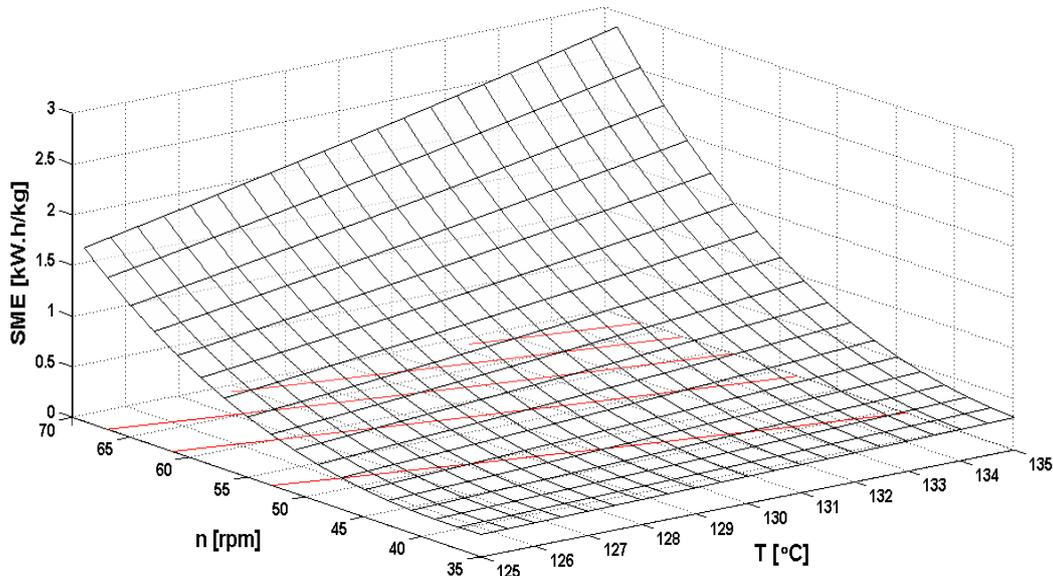
Fig. 8: Effect of screw speed and temperature on the SME requirement during extrusion process.
