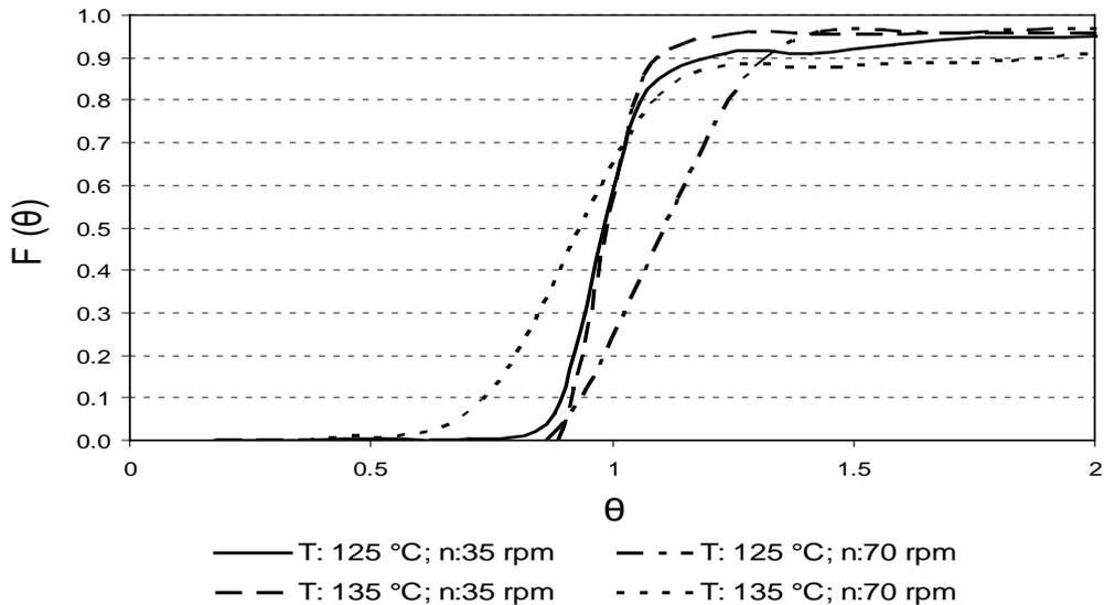
Fig. 7: Cumulative age distribution of acidified corn starch during extrusion process at the extreme operating conditions.
