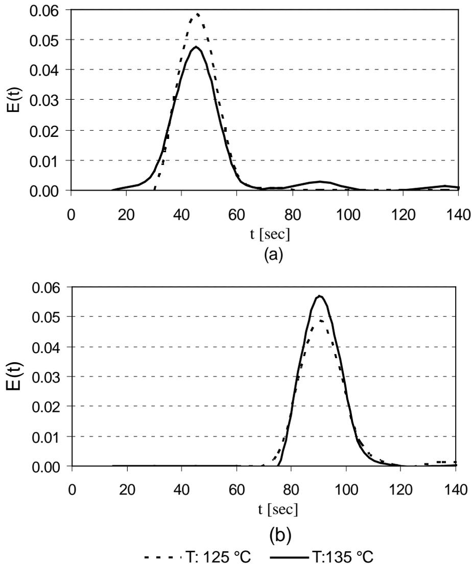
Fig. 6: Exit age distribution ( $E(t)$ ) of acidified corn starch during extrusion process at the extreme operating conditions where (a) at screw speed of 70 rpm, and (b) at screw speed of 35 rpm.
