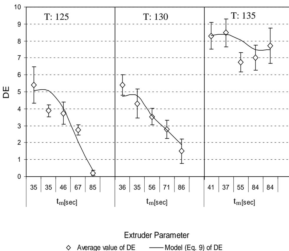
Fig. 5: Effect of mean residence time on the dextrose equivalence of dextrin during extrusion process, vertical error bars represent 95% confidence interval.
