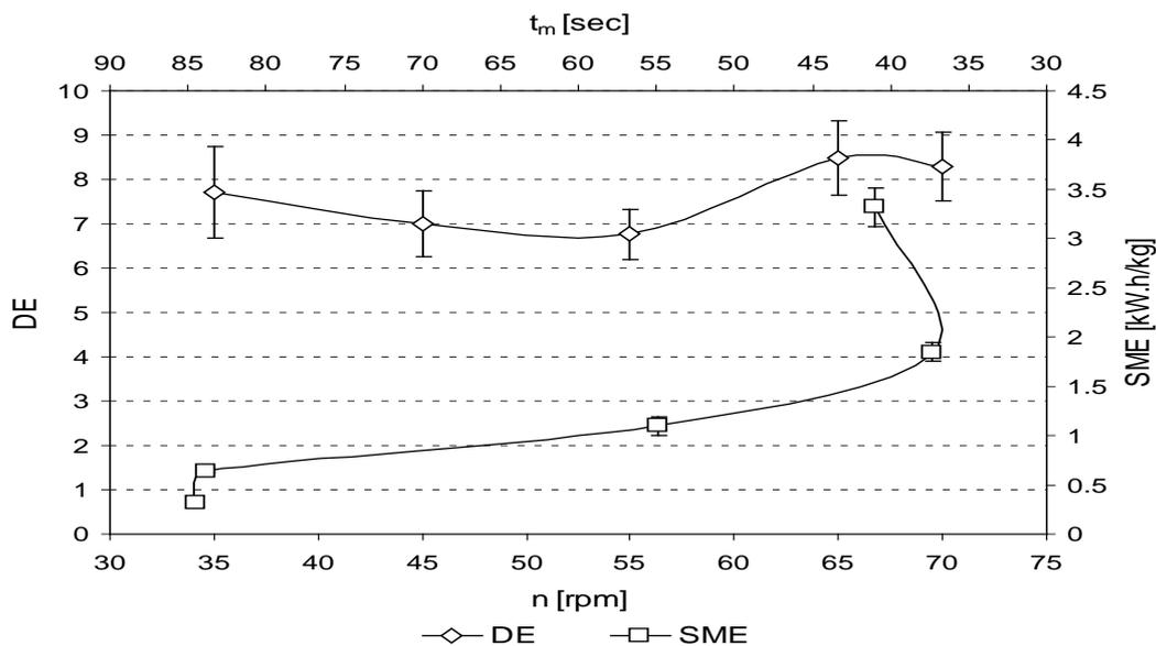
Fig. 10: Extrusion parameters at the best operating temperature (135 °C) as related to the dextrose equivalent of dextrin during extrusion process.
