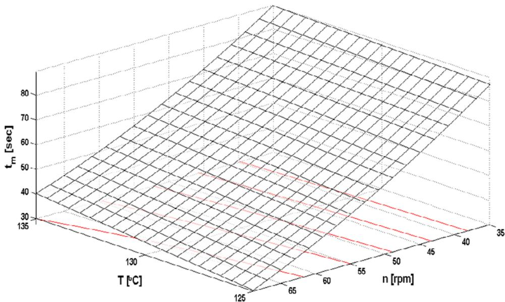
Fig. 4: Effect of screw speed and roasting temperature on the mean residence time of acidified corn starch during the extrusion process.
