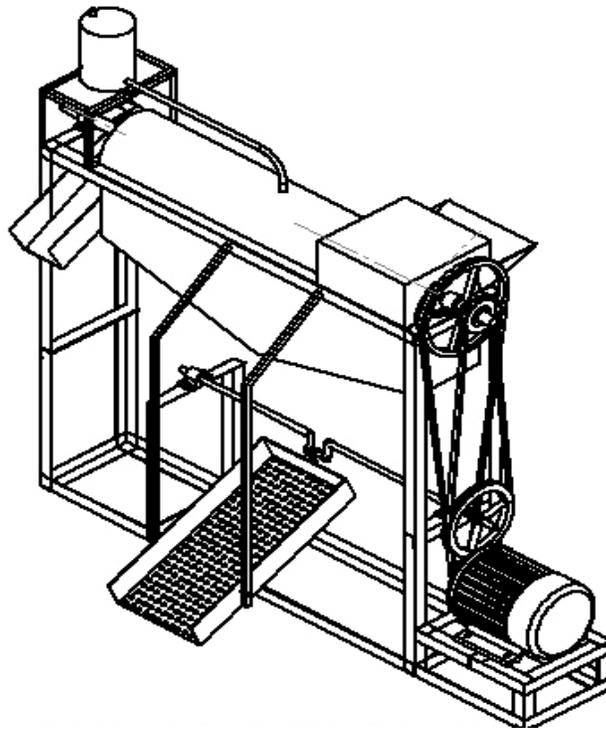
Fig. 3: Isometric View of the Melon Seed Extractor
