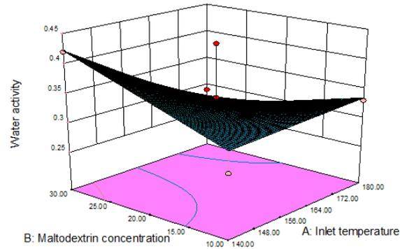
Fig. 2: Response surface plot showing relation between the moisture content (up) and water activity (down) as affected by inlet temperature and maltodextrin concentration.
