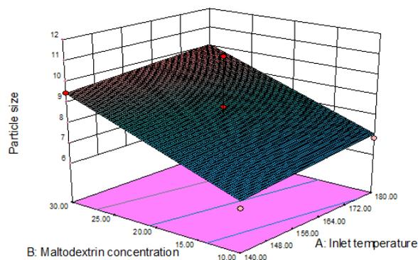
Fig. 4: Response surface plot showing relation between particle size as affected by inlet temperature and maltodextrin concentration.
