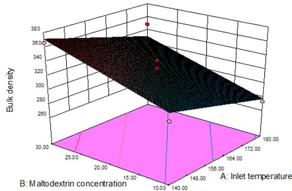
Fig. 3: Response surface plot showing relation between bulk density as affected by inlet temperature and maltodextrin concentration.
