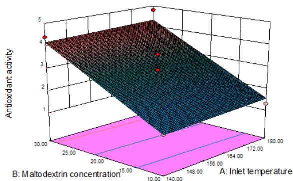
Fig. 6: The graphical presentation of regression equation showing the relation between the antioxidant activity as affected by inlet temperature and maltodextrin concentration.
