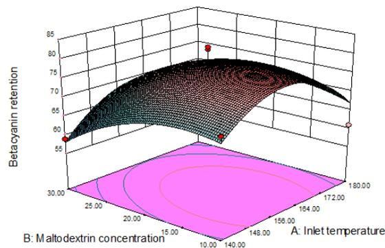
Fig. 1: Response surface plot showing relation between the betacyanin retention as affected by inlet temperature and maltodextrin concentration.
