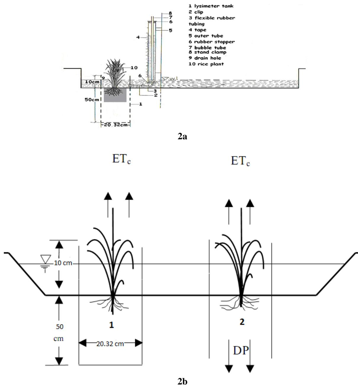
Fig 2 a, b: Cross-section of installed microlysimeter
