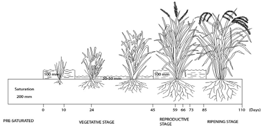
Fig 3: Water level for paddy at different growth stages [22]
