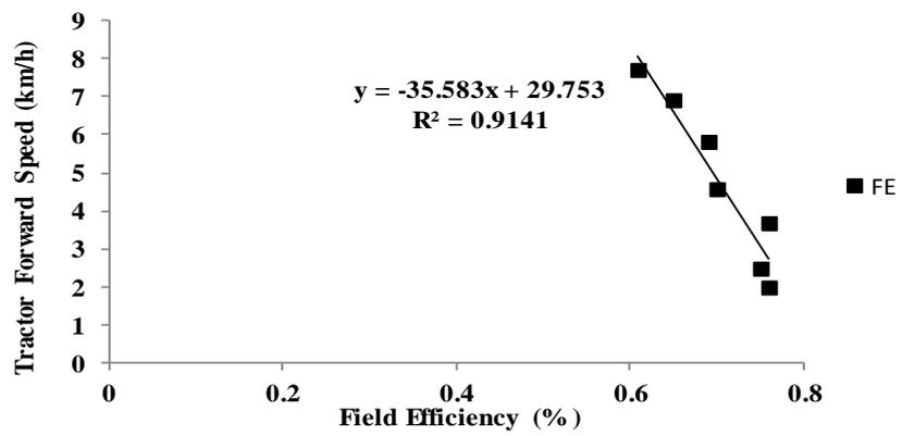
Fig. 5: Effect of speed on field efficiency
