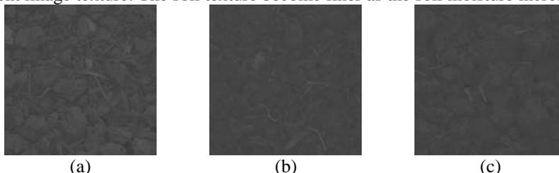
Fig. 2: Image of soil in grayscale. (a) MC=12% (b) MC=30% (c) MC=50%
