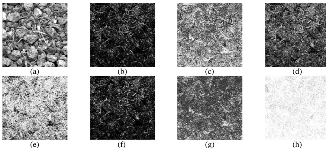
Fig. 3: Image of soil in different texture parameter. (a) mean (b) variance (c) homogeneity (d) dissimilarity (e) entropy (f) contrast (g) second moment (h) correlation
