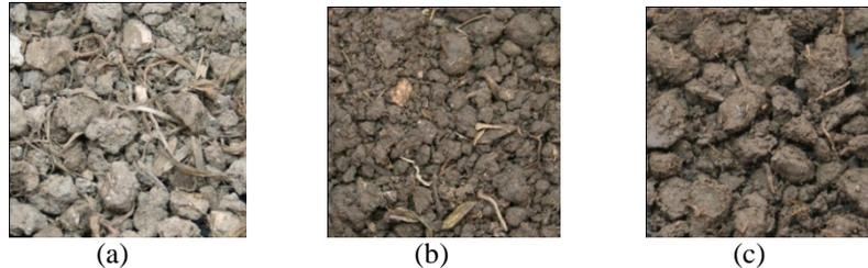
Fig. 1: Image of soil in RGB color. (a) MC=12% (b) MC=30% (c) MC=50%
