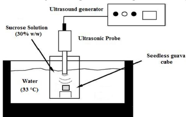
Fig. 1: Experimental set-up for ultrasonic treatment.
