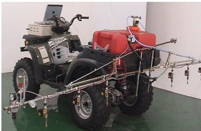
Fig. 3: Automatic Sprayer Installed with Web Camera and Communication Devices.
