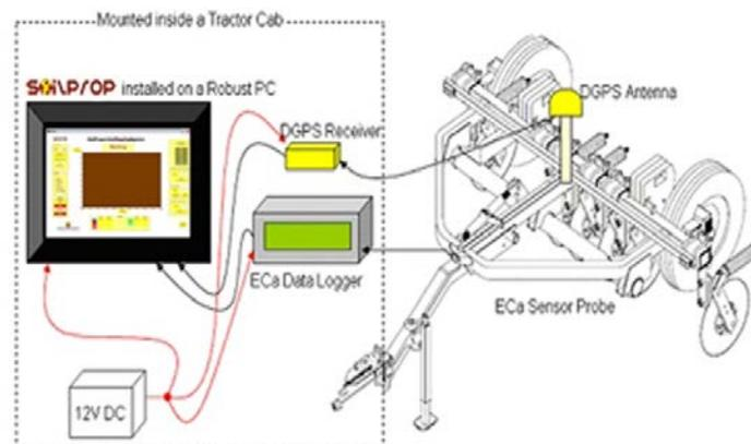
Fig. 4: The diagram of the developed system which comprising of various devices
