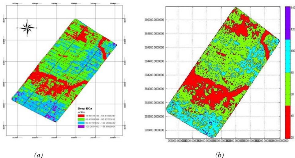
Fig. 6: Kriging map of soil ECad produced from ArcGIS 9.2 (a) and from the developed system (b) for 118 lots of the study area
