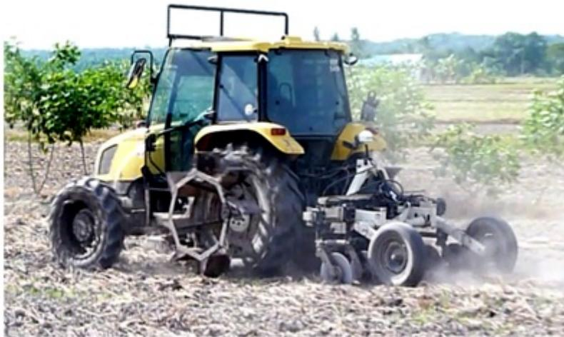
Fig. 2: Soil ECa sensor integrated with Trimble Ag132 DGPS pulled by a tractor
