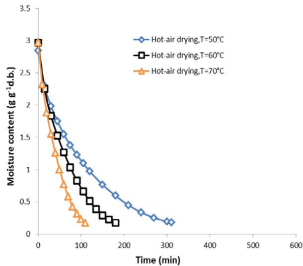
Fig. 5: Hot-air drying moisture removal for banana slices.
