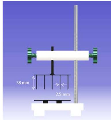
Fig. 1: A schematic of the multiple points to plate electrohydrodynamic (EHD) system.
