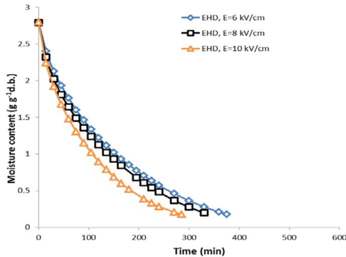
Fig. 3: Electrohydrodynamic (EHD) moisture removal for banana slices.
