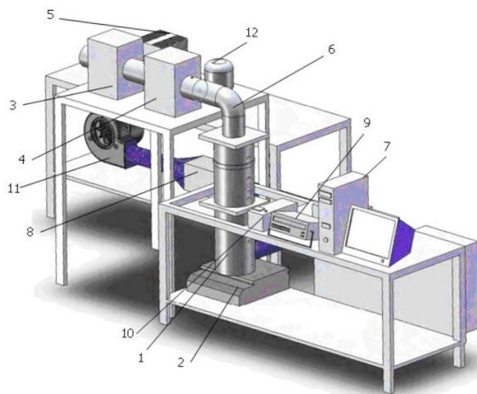
Fig. 2: A schematic of the convective hot-air dryer setup: (1) drying chamber, (2) digital scale, (3) condenser, (4) evaporator, (5) external condenser, (6) flexible tube, (7) PC, (8) electrical heater, (9) digital multi-meter, (10) frequency inverter, (11) centrifugal fan and (12) compressor.
