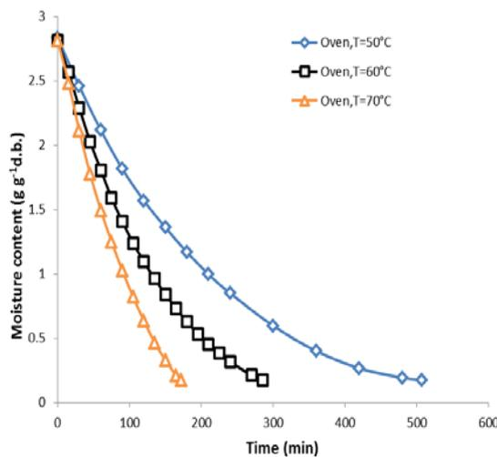
Fig. 4: Oven drying moisture removal for banana slices.
