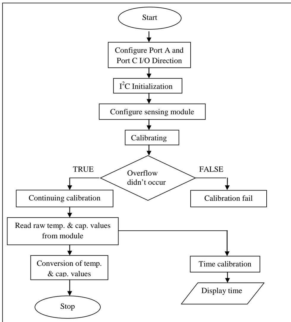
Fig. 3: Programing Flow Chart for Capacitance Measurement and CPO Contamination Detection
