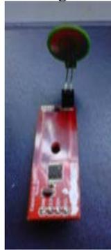
Fig. 1: Sensor Head for AD7746 Capacitance to Digital Converter
