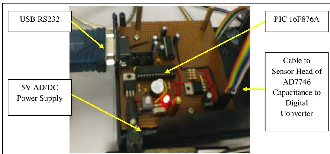
Fig. 2 : Circuit board for capacitance measurement using AD7746 Capacitance to Digital Converter
