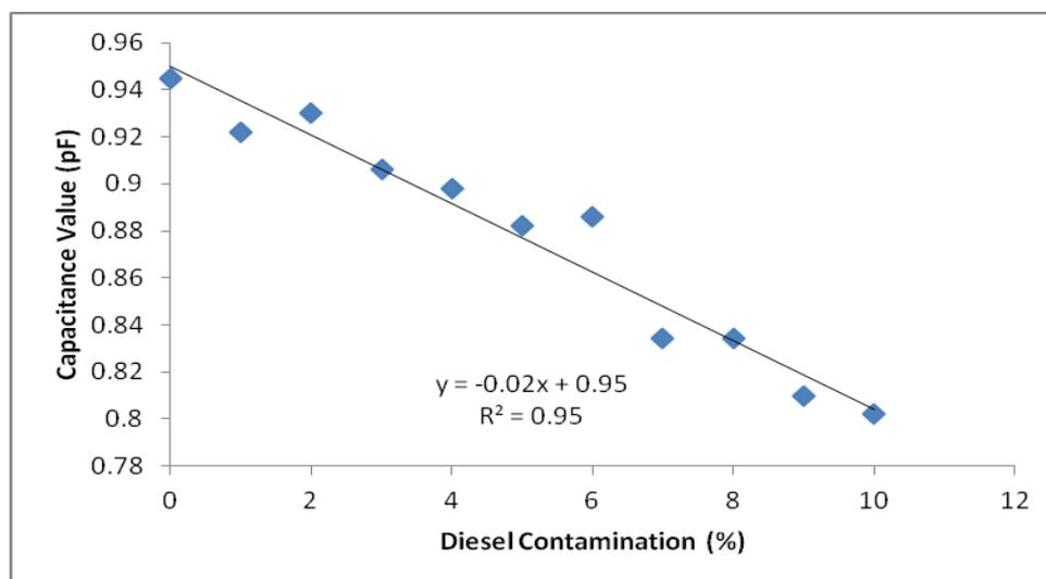
Fig. 5 : Capacitance value of CPO versus diesel contamination levels (0-10)% contamination with linear regression model ( $r^2=0.95$ )
