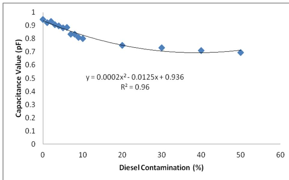
Fig. 4 : Capacitance value of CPO versus diesel contamination levels (0-50)% contamination.
