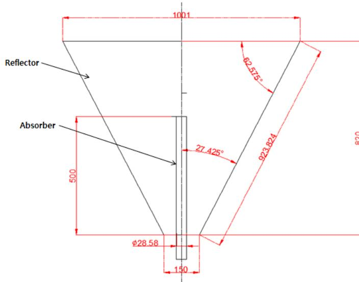
Figure 1. Drawing of conical solar collector.
