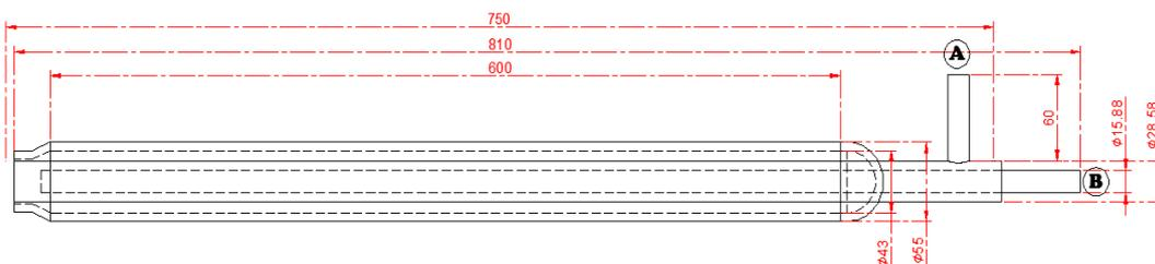
Figure 3. Drawing of CTA with glass tube.
