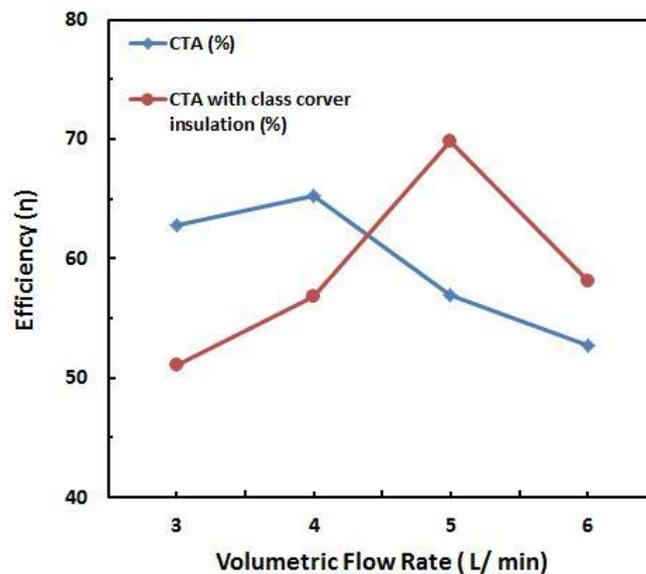
Figure 5. Comparison of efficiency with and without glass tube.
