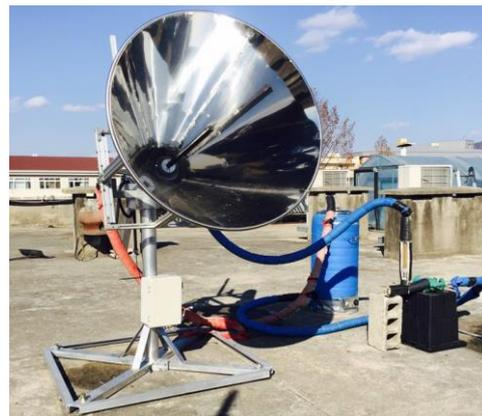
Figure 4. Configuration and photograph of conical solar collector.
