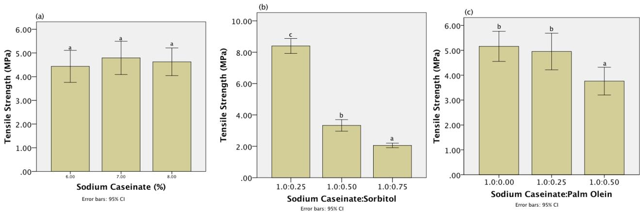
Figure 2. Changes of Tensile Strength of Sodium Caseinate Edible Films with (a) sodium caseinate at different concentration, (b) sorbitol at different concentration, and (c) palm olein at different concentration.
