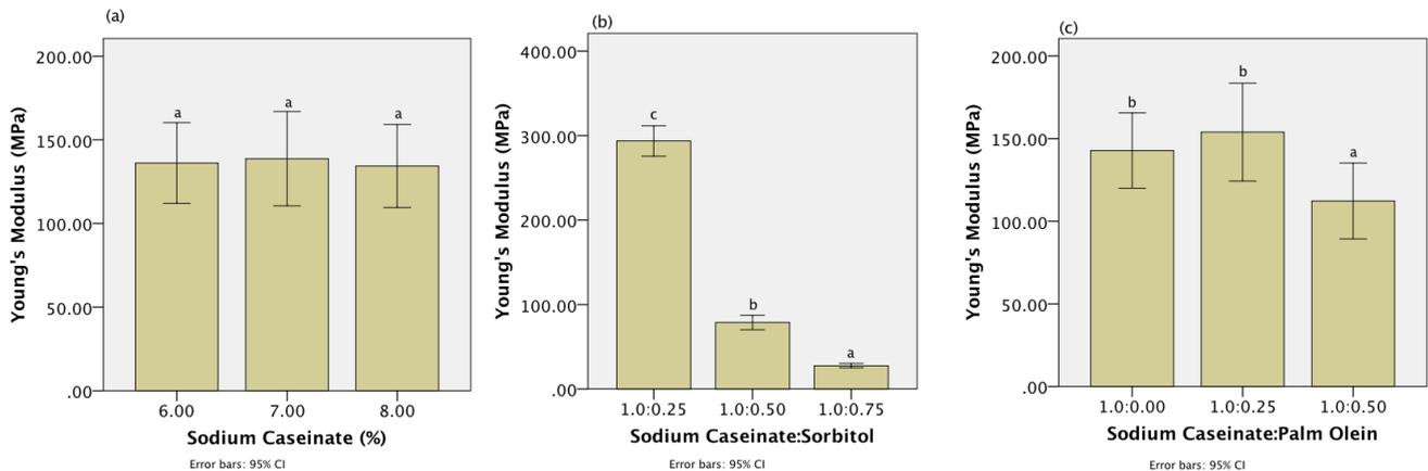
Figure 4. Changes of Young's Modulus of Sodium Caseinate Edible Films with (a) sodium caseinate at different concentration, (b) sorbitol at different concentration, and (c) palm olein at different concentration.
