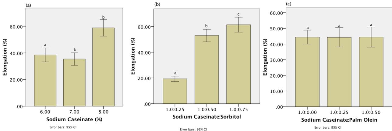
Figure 3. Changes of Percentage of Elongation of Sodium Caseinate Edible Films with (a) sodium caseinate at different concentration, (b) sorbitol at different concentration, and (c) palm olein at different concentration.
