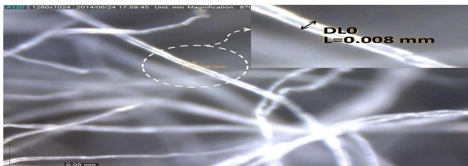
Figure 1. Size of bleached Kenafbast fibre under Dino-Lite (200 X).
