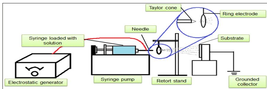
Figure 2. The setup of electro-spray.
