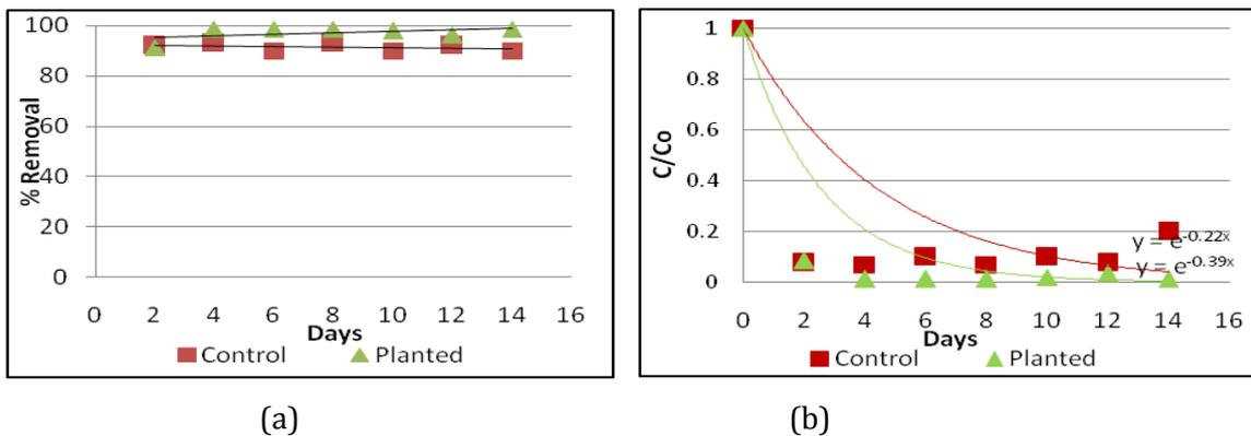
Figure 3. (a) Ammonia Nitrogen ( $\text{NH}_3\text{-N}$ ) removal efficiency (b) Performance of removal analysis.
