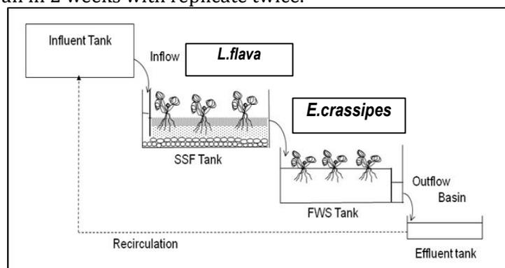
Figure 1. Experiment setup of SSF-FWS CW systems.
