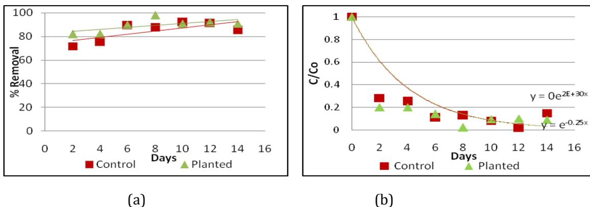
Figure 4. Nitrate ( $\text{NO}_3\text{-N}$ ) removal efficiency (b) Performance of removal analysis.
