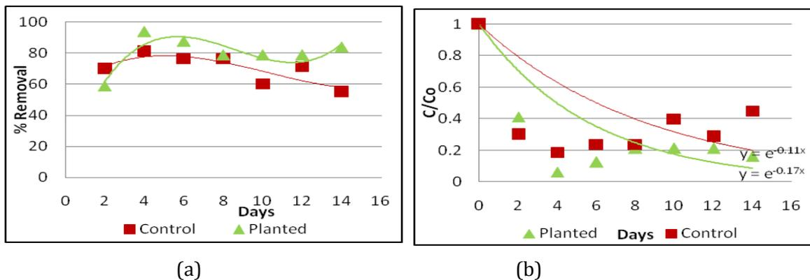
Figure 2. (a) COD removal efficiency (b) Performance of COD removal analysis
