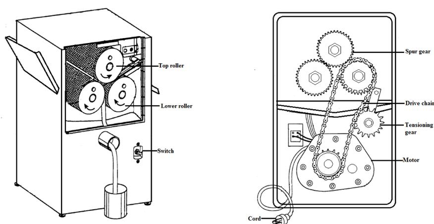
Figure 1. Schematic diagram of sugarcane press machine
