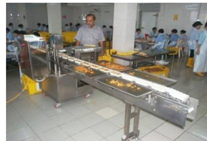
Figure 2. Automatic satay skewing machine.
