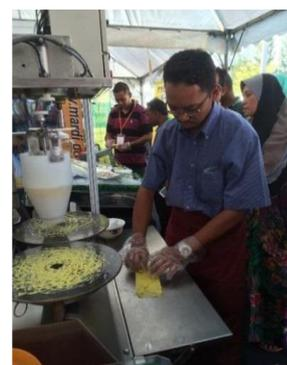
Figure 10. *Kuih roti jala* forming machine.
