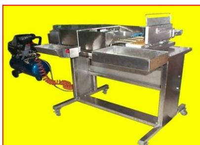
Figure 3. Semi-automatic satay skewing machine.
