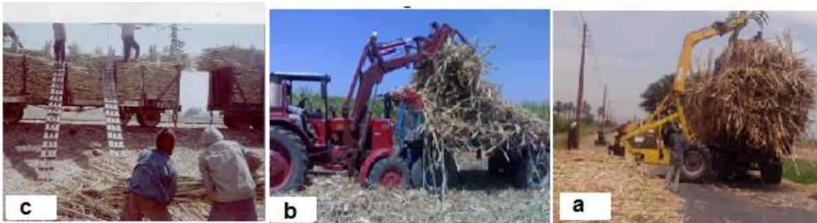
Figure 1. Sugarcane loading a) self propelled loader in site, b) Tractor mounted loader in site and c) Labor loading in site.
