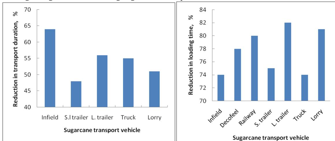
Figure 4. Reduction of loading and transport duration due to mechanical loading.
