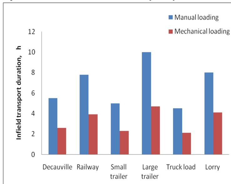
Figure 2. Infield transport duration required to handle the full load of sugarcane to main transport vehicles.
