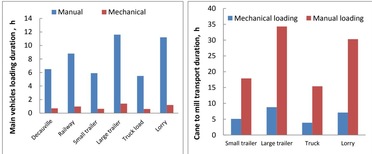
Figure 3. Main vehicle loading and transport duration.
